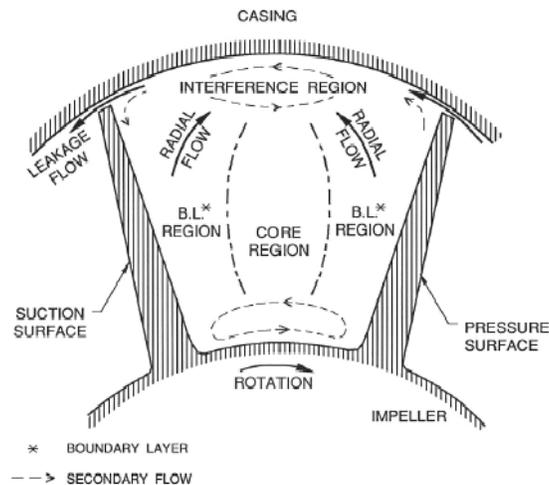
Figure 1: Cross-section of a blade passage in an axial flow impeller showing the tip leakage flow, boundary layer radial flow, and other secondary flows (adapted from Lakshminarayana 1981).
