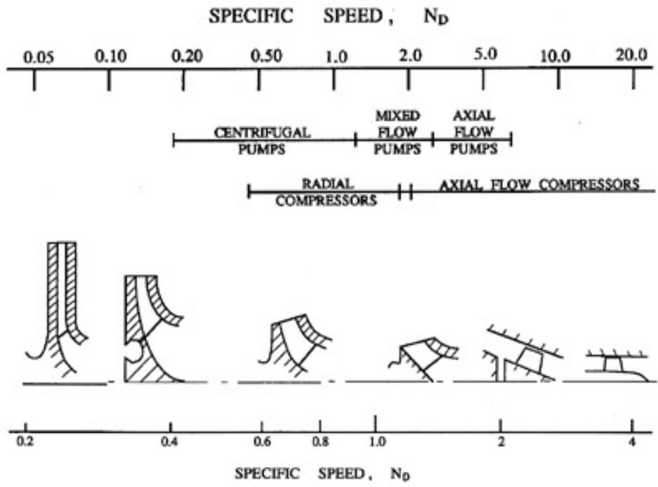
Figure 2: Pump shapes as a function of the specific speed,  $N$  (from Sabersky, Acosta and Hauptmann 1989).
