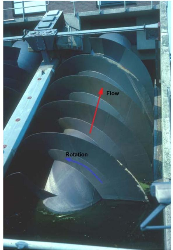
Figure 1: Left: Ancient Persian water wheel. Right: An Archimedes screw used to lift water in Netherlands from one canal to another.
