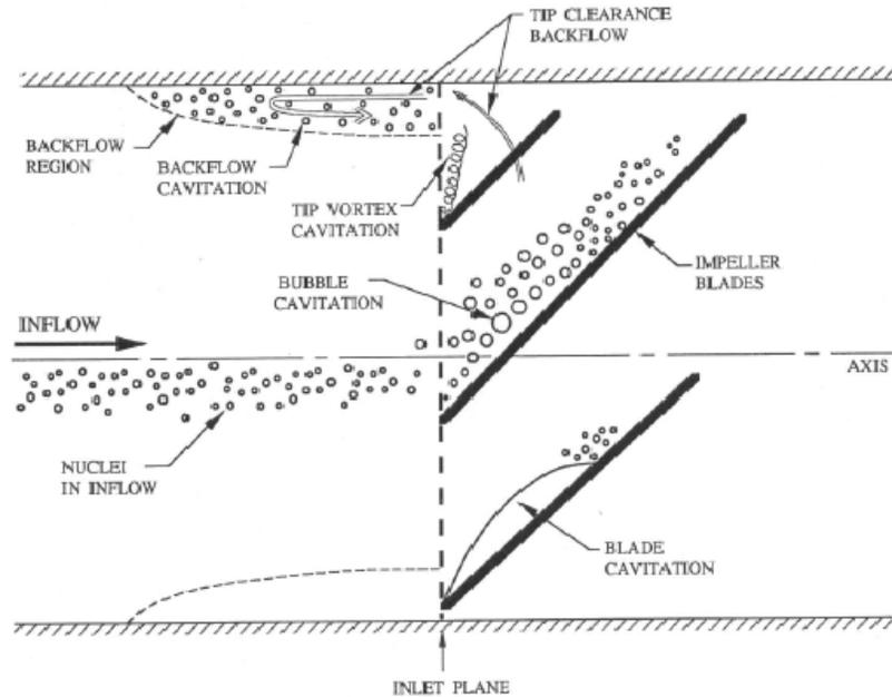
Figure 1: Types of cavitation in pumps.
