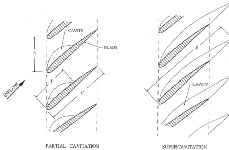
Figure 5: Partially cavitating cascade (left) and supercavitating cascade (right).
