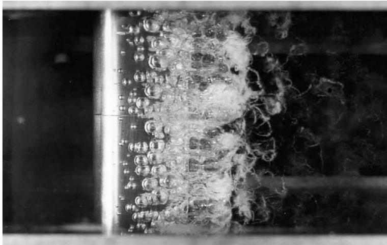
Figure 3: Bubble cavitation on the surface of a NACA 4412 hydrofoil at zero incidence angle, a speed of 13.7 *m/s* and a cavitation number of 0.3. The flow is from left to right and the leading edge of the foil is just to the left of the white glare patch on the surface (Kermeen 1956).
