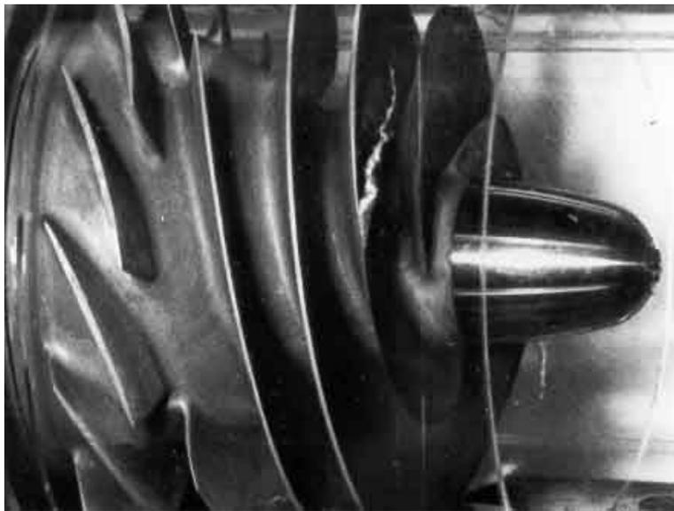
Figure 2: Tip vortex cavitation on Impeller IV, the scale model of the SSME low pressure LOX turbopump (see figure ??) at an inlet flow coefficient,  $\phi_1$ , of 0.07 and a cavitation number,  $\sigma$ , of 0.42 (from Braisted 1979).
