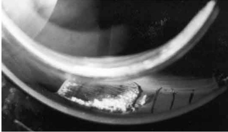
Figure 4: Blade cavitation on the suction surface of a blade in a centrifugal pump. The relative flow is from left to right and the cavity begins at the leading edge of the blade which is toward the left of the photograph. From Sloteman, Cooper, and Graf (1991), courtesy of Ingersoll-Dresser Pump Company.
