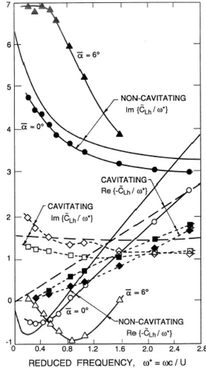
Figure 1: Fluctuating lift coefficient,  $\tilde{C}_{Lh}$ , for foils undergoing heave oscillations at a reduced frequency,  $\omega^* = \omega c / U$ . Real and imaginary parts of  $\tilde{C}_{Lh} / \omega^*$  are presented for (a) non-cavitating flow at mean incidence angles of  $0^\circ$  and  $6^\circ$  (b) cavitating data for a mean incidence of  $8^\circ$ , for very long choked cavities ( $\square$ ) and for cavities 3 chords in length ( $\diamond$ ). Adapted from Acosta and DeLong (1971).
