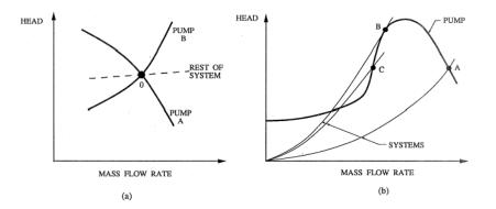
Figure 1: Quasistatically stable and unstable operation of pumping systems.
