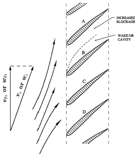
Figure 1: Schematic of a stall cell in rotating stall or rotating cavitation.
