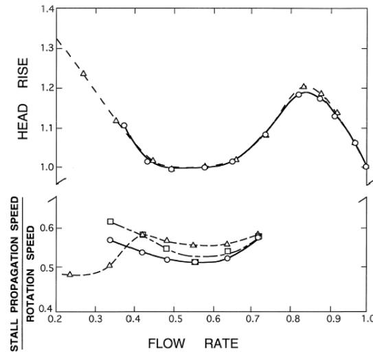
Figure 2: The head characteristic for an 18-bladed axial flow pump along with the measurements of the propagation velocity of the rotating stall cell relative to the shaft speed. Adapted from Murai (1968). Data is shown for three different inlet pressures. Flow and head scales are dimensionless.
