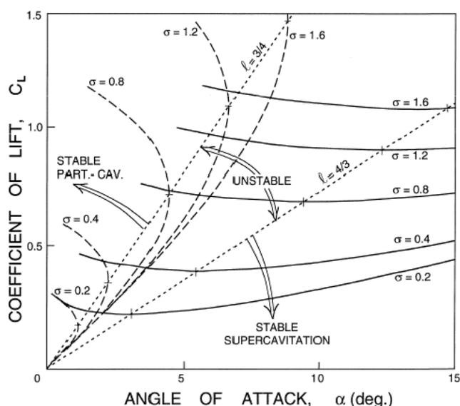
Figure 1: The lift coefficient for a flat plate from the partial cavitation analysis of Acosta (1955) (dashed lines) and the supercavitating analysis of Tulin (1953) (solid lines);  $C_L$  is shown as a function of angle of attack,  $\alpha$ , for several cavitation numbers,  $\sigma$ . The dotted lines are the boundaries of the region in which the cavity length is between  $3/4$  and  $4/3$  of a chord, and in which  $dC_L/d\alpha < 0$ .
