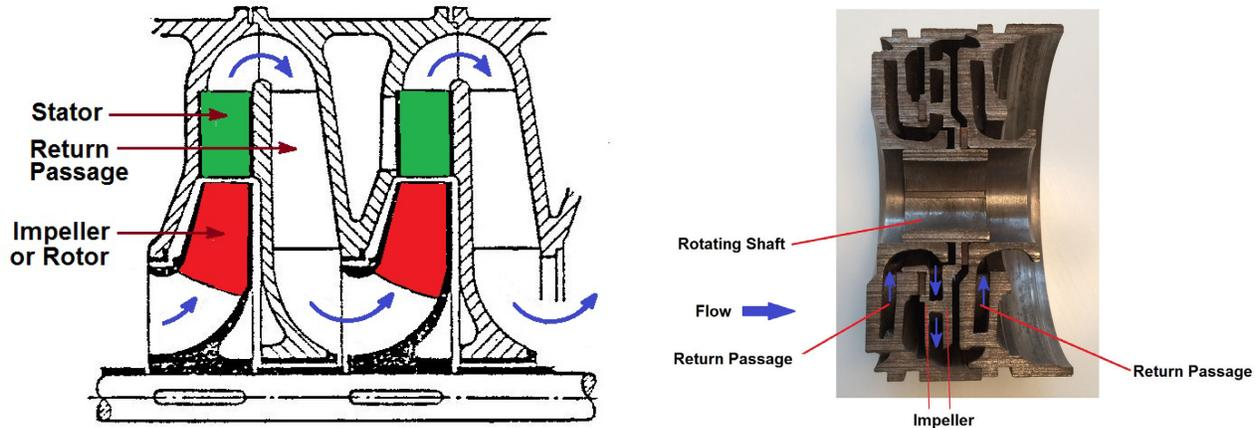
Figure 1: Left: Typical multistage centrifugal pump. Right: One stage of a down-hole oil well pump.
