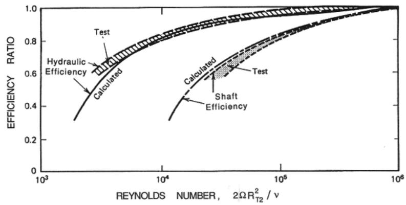
Figure 11: The dependence of hydraulic efficiency,  $\eta_P$ , and shaft efficiency,  $\eta_S$ , on Reynolds number,  $2\Omega R_{T2}^2/\nu$  (from Balje 1981).
