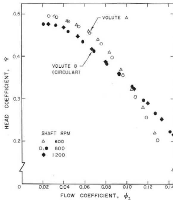
Figure 3: Typical non-cavitating performance for a centrifugal pump, namely Impeller X (see section (Mbbi)) with Volute A and a circular volute of uniform cross-section (from Chamieh 1983).
