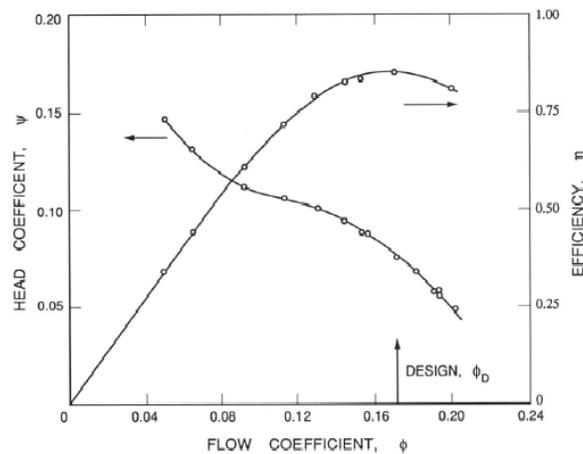
Figure 5: Typical non-cavitating performance characteristics for a 20.3cm diameter, 3-bladed axial flow pump with a hub-tip ratio,  $R_H/R_T$ , of 0.45 running at about 1500rpm. At the blade tip the chord is 7.3cm, the solidity is 0.344 and the blade angle,  $\beta_{bT}$ , is 11.9°. Adapted from Guinard *et al.* (1953).
