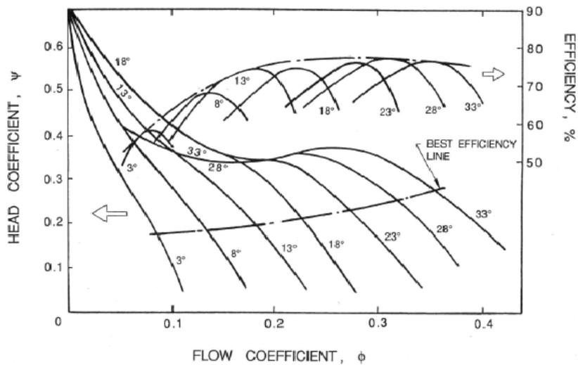
Figure 8: Head and efficiency characteristics for an axial flow pump with different tip blade angles,  $\beta_{bT}$  (from Peck 1966).
