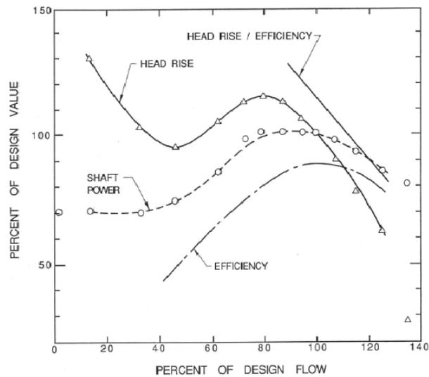
Figure 7: Characteristics of a mixed flow pump (Myles 1966).
