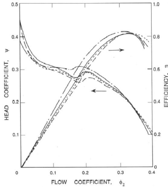
Figure 6: Typical non-cavitating performance characteristics for a four-bladed axial flow pump with tip blade angle,  $\beta_{bT}$ , of about  $18^\circ$ , a hub-tip ratio,  $R_H/R_T$ , of 0.483, a solidity of 0.68 and four different blade profiles (yielding the set of four performance curves). Adapted from Oshima and Kawaguchi (1963).
