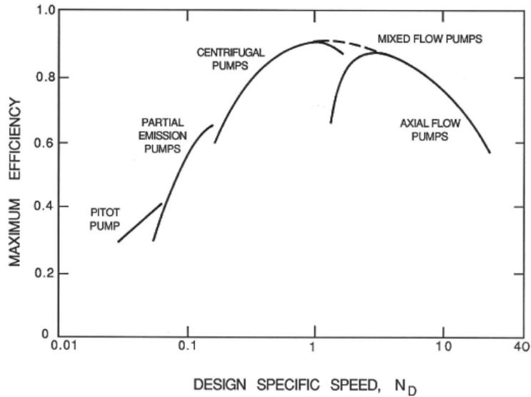
Figure 10: Compilation by Balje (1981) of maximum efficiencies for various kinds of pumps as a function of design specific speed,  $N_D$ . Since efficiency is also a function of Reynolds number the data has been corrected to a Reynolds number,  $2\Omega R_{T2}^2/\nu$ , of  $10^8$ .
