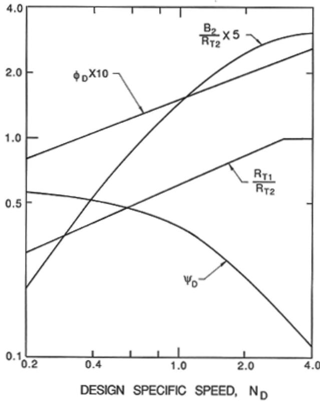
Figure 9: General design guidelines for pumps indicating the optimum ratio of inlet to discharge tip radius,  $R_{T1}/R_{T2}$ , and discharge width ratio,  $B_2/R_{T2}$ , for various design specific speeds,  $N_D$ . Also shown are approximate pump performance parameters, the design flow coefficient,  $\phi_D$ , and the design head coefficient,  $\psi_D$  (adapted from Sabersky, Acosta and Hauptmann 1989).
