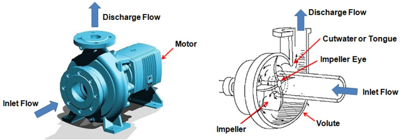
Figure 2: Examples of centrifugal pumps.
