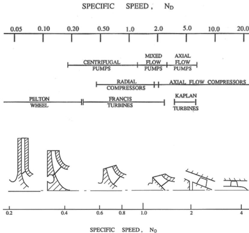
Figure 1: Typical turbomachine geometries for a range of specific speeds (from Sabersky, Acosta and Hauptmann 1989).
