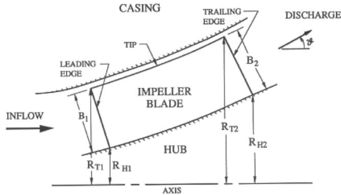
Figure 1: Cross-sectional view through the axis of a pump impeller.
