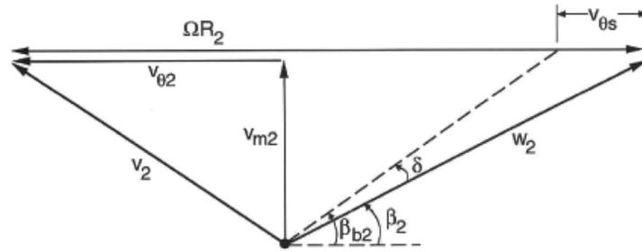
Figure 4: Velocity vectors at discharge indicating the slip velocity,  $v_{\theta s}$ .
