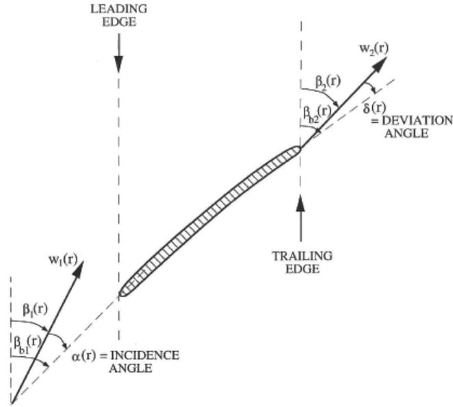
Figure 3: Repeat of figure 2 showing the definitions of the incidence angle at the leading edge and the deviation angle at the trailing edge.
