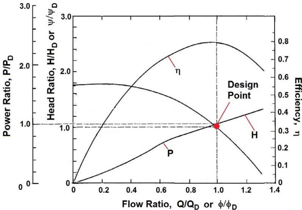
Figure 2: An example of a set of dimensionless pump characteristics, in the case of a  $R_{T2} = 0.178m$  centrifugal pump with a specific speed,  $N_D = 0.8$ , and a discharge blade angle,  $\beta_{b2} = 23^\circ$ . Adapted from Karassik *et al* (1986).
