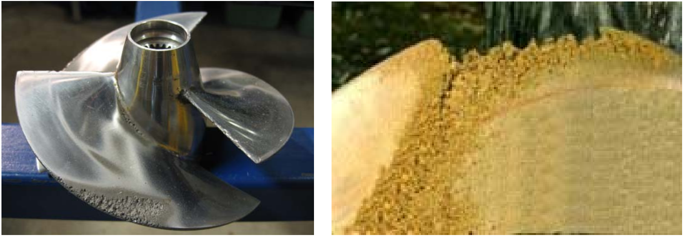
Figure 1: Left: Typical cavitation damage to the stainless steel ducted propeller from a personal watercraft. Right: Close-up of cavitation damage to a marine propeller tip.
