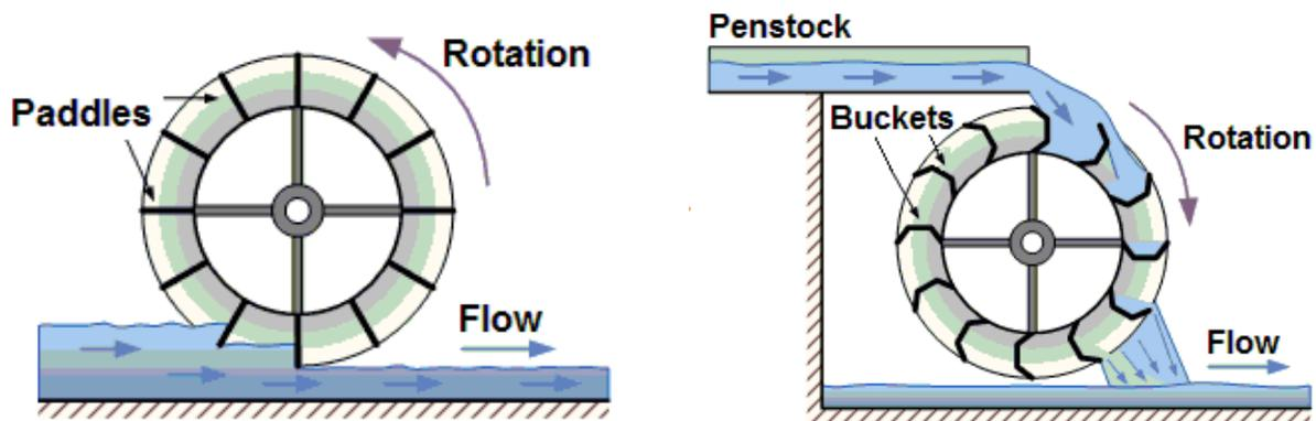
Figure 1: Undershot (left) and overshot (right) water wheels.
