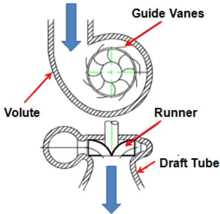
Figure 4: Schematic of a Francis turbine.
