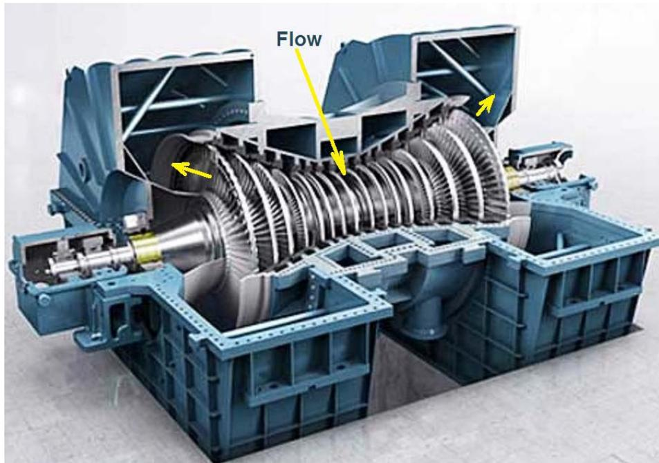
Figure 6: Schematic of an axial flow steam turbine.
