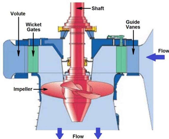
Figure 3: Schematic of a propeller turbine or Kaplan turbine.
