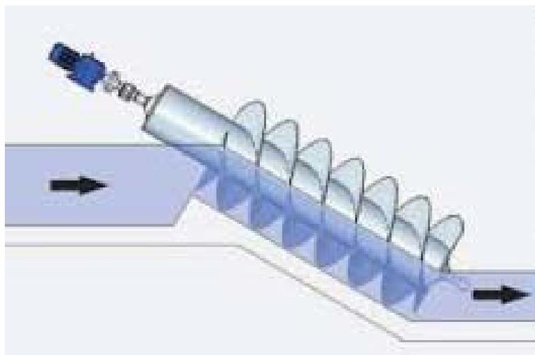
Figure 5: Schematic of an Archimedes turbine.
