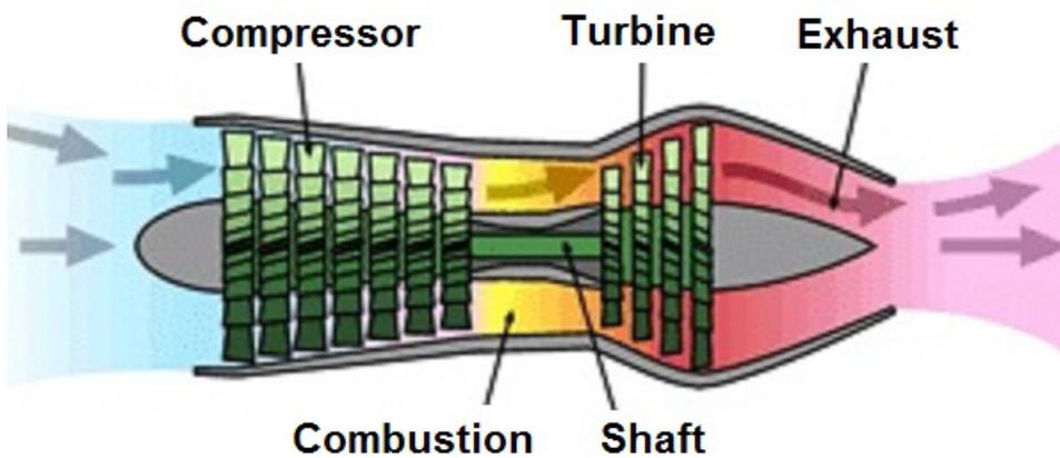
Figure 7: Schematic of a typical jet engine.
