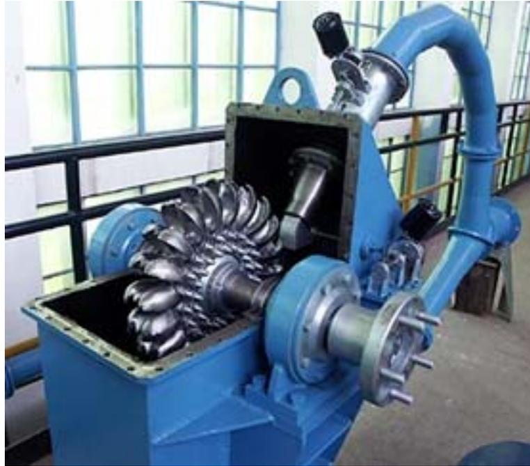
Figure 2: Pelton wheel turbine.
