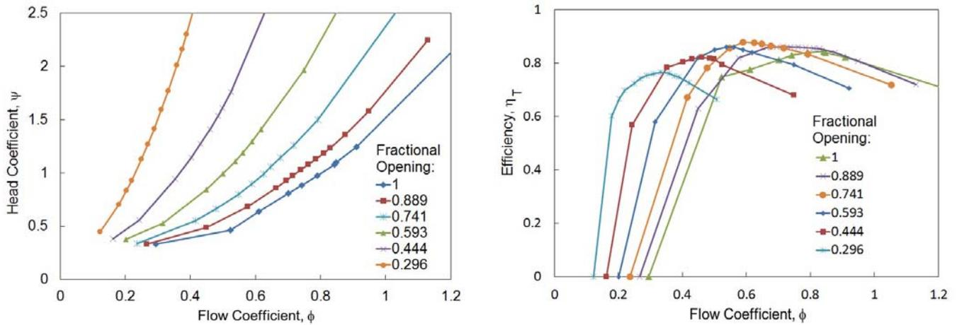
Figure 1: Head Coefficient,  $\psi$ , and efficiency,  $\eta_T$ , for a  $R_{T1} = 16in$  Wellman-Seaver-Morgan reaction turbine at a series of gate openings (data from Daugherty (1920)).
