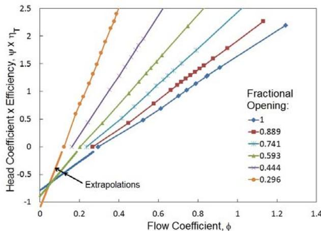
Figure 2: Head Coefficient,  $\psi$ , multiplied by the efficiency,  $\eta_T$ , for the data of Figure 1.
