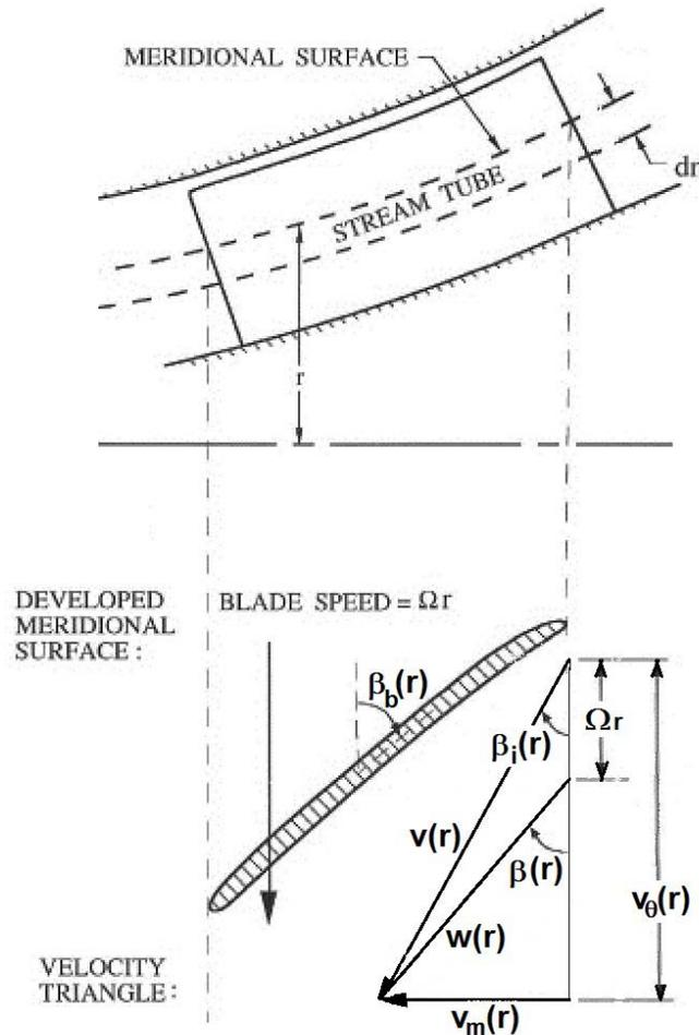
Figure 1: Developed meridional surface and velocity triangle.
