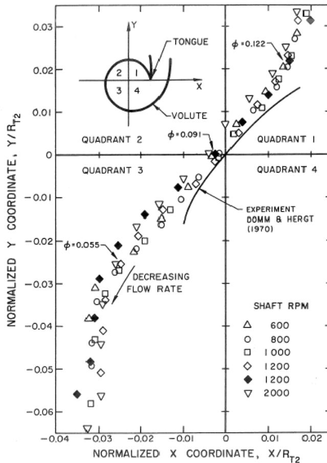
Figure 5: Locus of the zero radial force locations for the Impeller X/Volute A combination (Chamieh *et al.* 1985) compared with that from the data of Domm and Hergt (1970).
