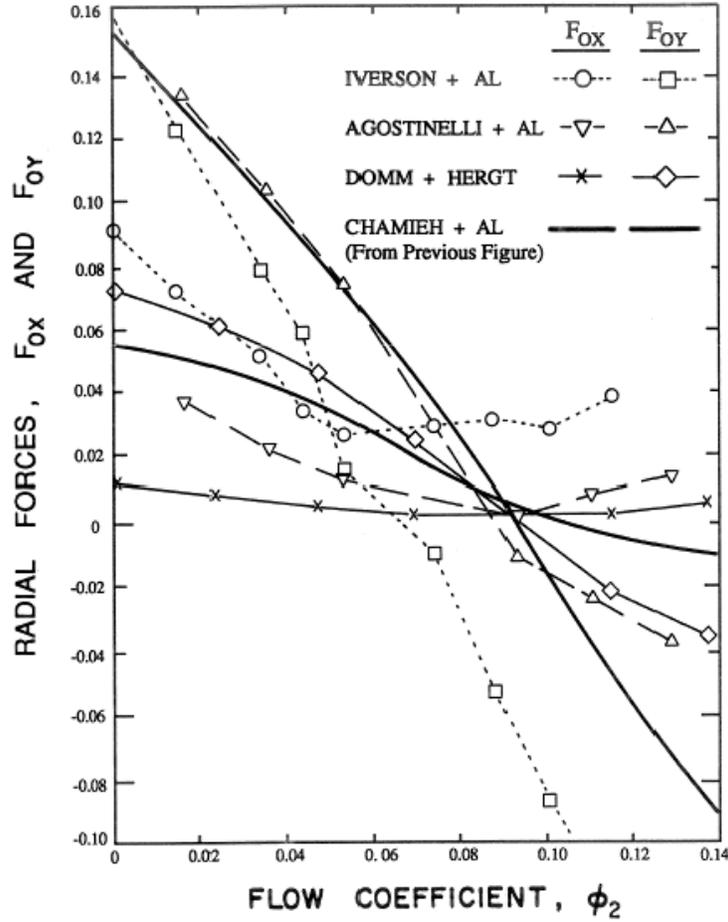
Figure 2: Comparison of the radial forces measured by Iverson, Rolling and Carlson (1960) on a pump with a specific speed,  $N_D$ , of 0.36, by Agostinelli, Nobles and Mockeridge (1960), on a pump with  $N_D = 0.61$ , by Domm and Hergt (1970), and by Chamieh *et al.* (1985) on a pump with  $N_D = 0.57$ .
