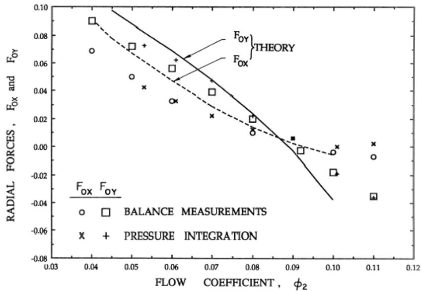
Figure 8: Comparison of radial forces from direct balance measurements, from integration of measured pressures, and from theory for the Impeller X/Volute A combination (from Adkins and Brennen 1988).
