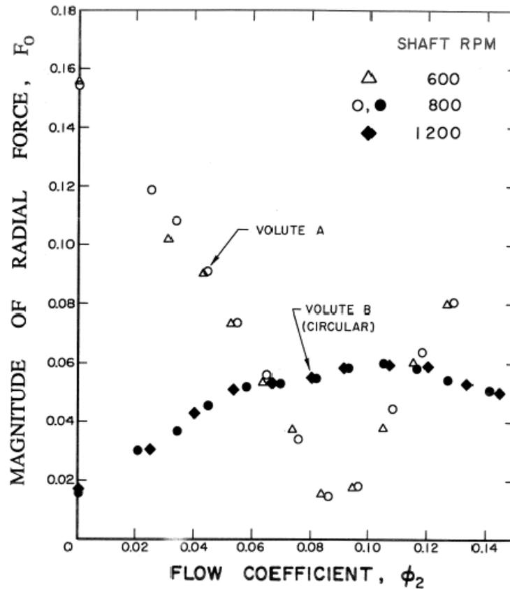
Figure 3: Comparison of the magnitude of the radial force ( $F_0$ ) on Impeller X caused by Volute A and by the circular Volute B with a circumferentially uniform area (Chamieh *et al.* 1985).
