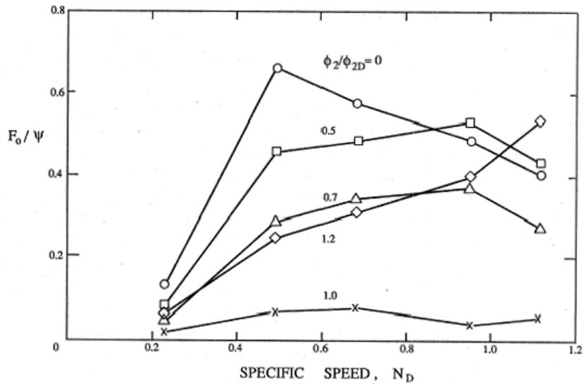
Figure 4: Variation of the radial force magnitude,  $F_0$ , divided by the head coefficient,  $\psi$ , as a function of specific speed,  $N_D$ , and flow for a class of volute casing pumps (adapted from KSB 1975).
