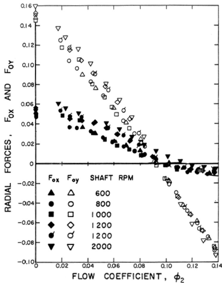
Figure 1: Radial forces for the centrifugal Impeller X/Volute A combination as a function of shaft speed and flow coefficient (Chamieh *et al.* 1985).
