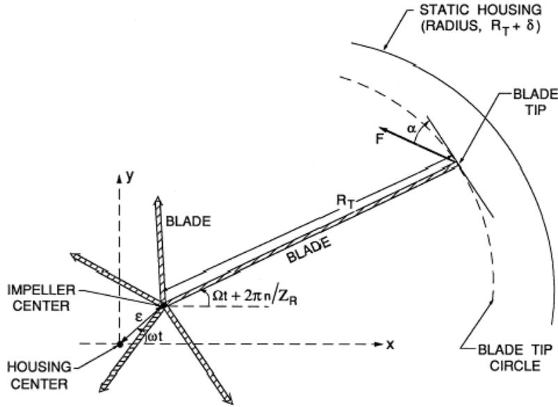
Figure 1: Schematic of the position of an axial flow turbomachine blade tip relative to a static housing as a result of the combination of rotational and whirl motion (details shown for only one of the  $Z_R$  blade tips).
