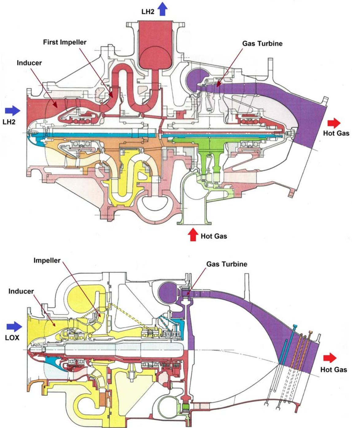
Figure 11: The liquid hydrogen (top) and liquid oxygen (bottom) pumps in the Ariane V rocket engine.
