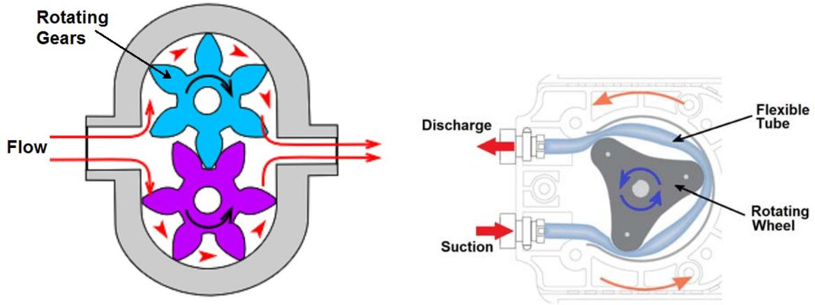
Figure 15: Left: Schematic of a typical gear pump. Right: Schematic of a typical peristaltic pump.
