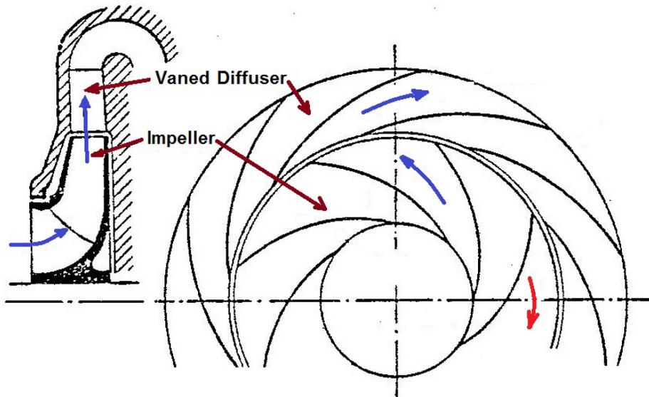
Figure 6: Typical centrifugal pump vaned diffuser.
