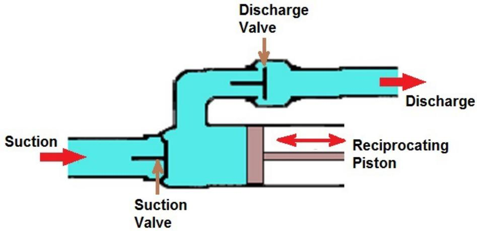
Figure 14: Schematic of a simple positive displacement pump.
