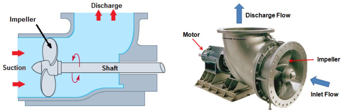
Figure 1: Schematic and picture of typical axial flow pumps.
