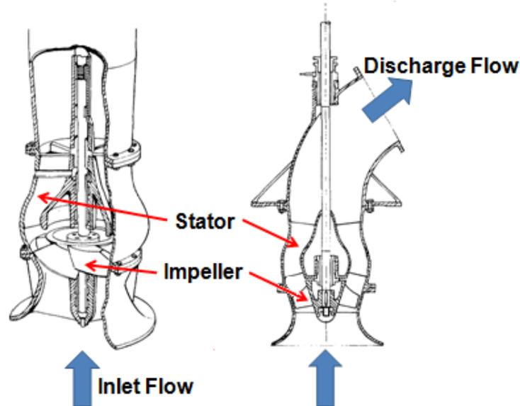
Figure 2: Typical mixed flow pump.
