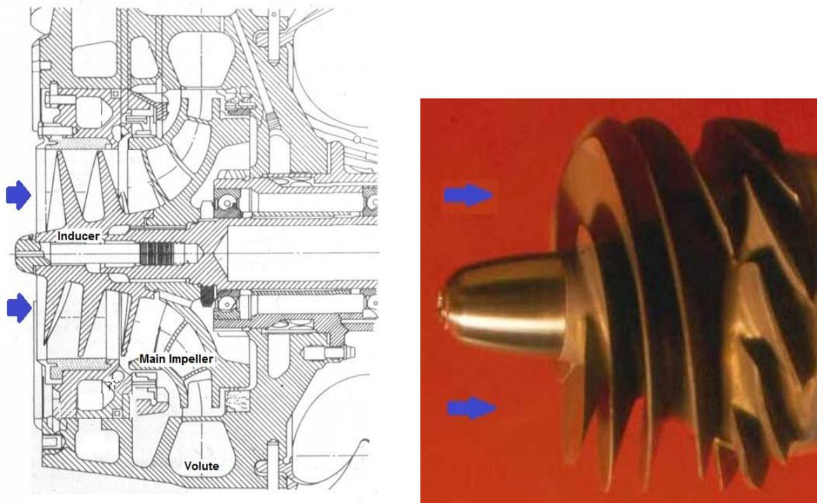
Figure 9: Left: The liquid oxygen pump in the J2 rocket engine. Right: Scale model of the low pressure liquid oxygen pump impeller in the Space Shuttle Main Engine.
