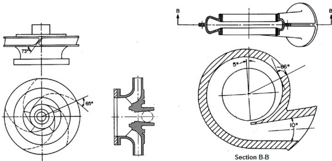
Figure 5: Typical centrifugal pump impeller (left) and volute (right).
