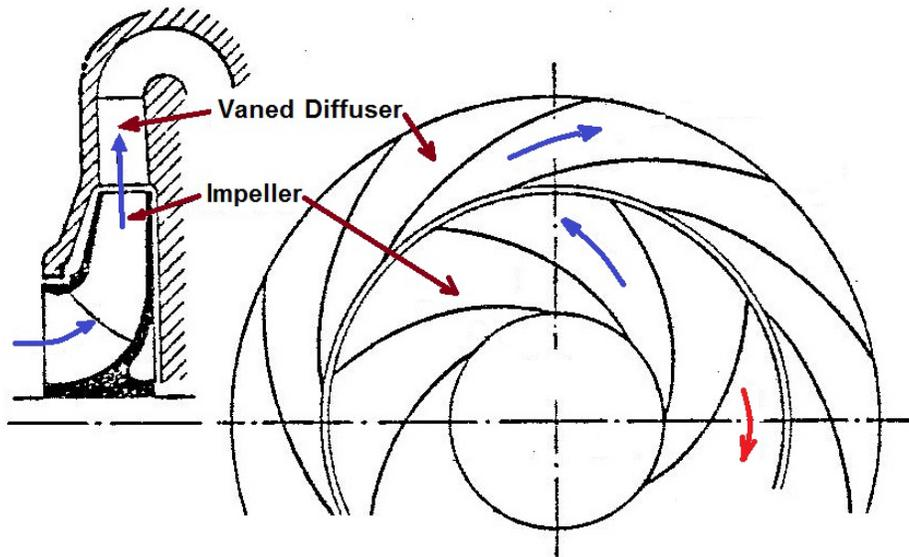
Figure 6: Typical centrifugal pump vaned diffuser.
