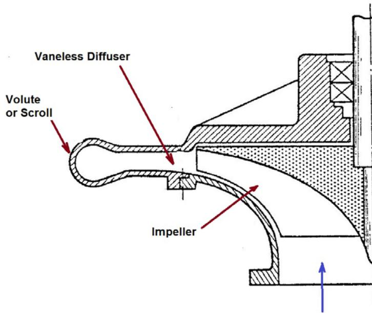
Figure 12: Typical centrifugal compressor.
