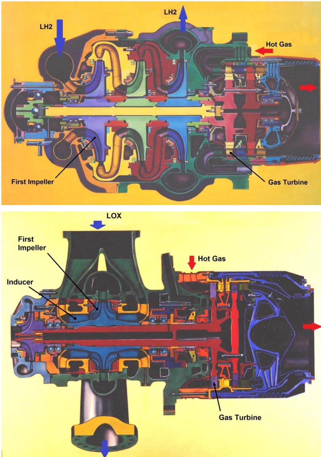
Figure 10: The high pressure liquid hydrogen (top) and liquid oxygen (bottom) pumps in the Space Shuttle Main Engine.
