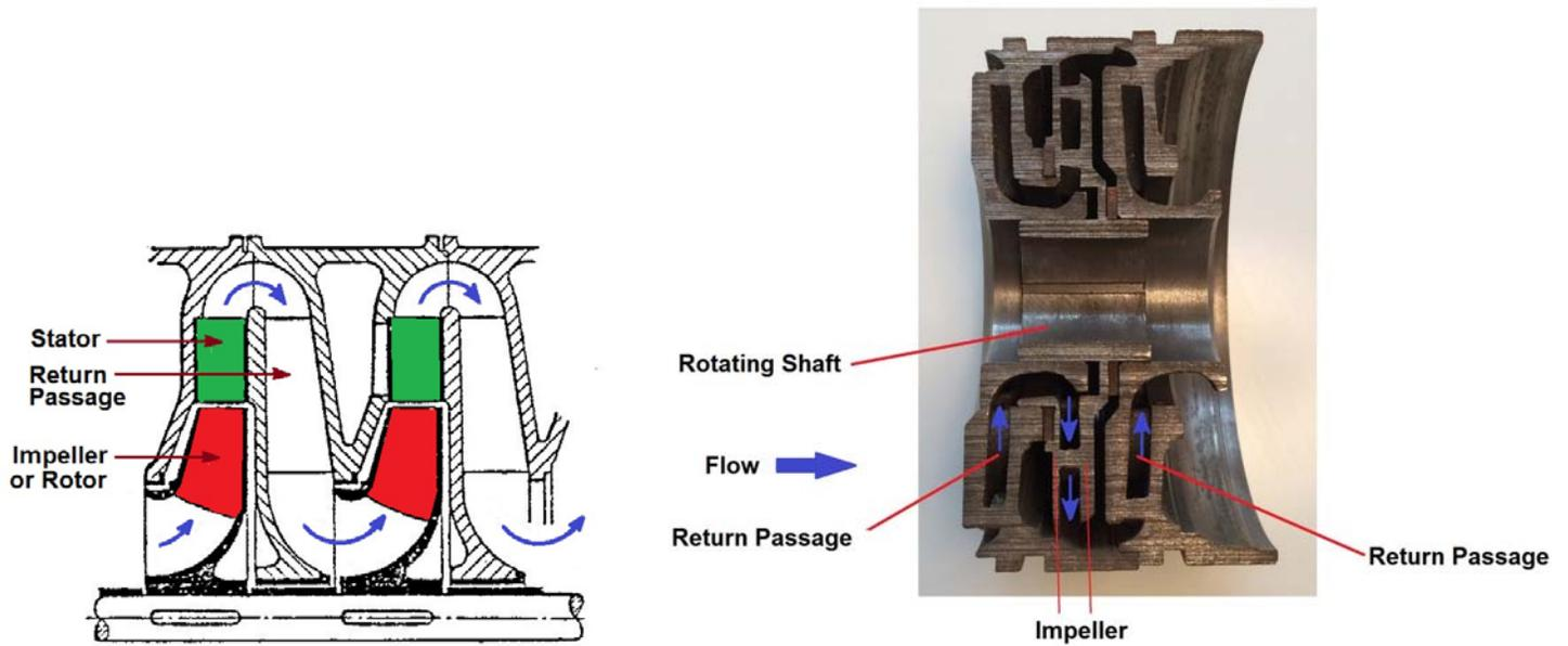
Figure 7: Left: Two-plus stages of a multistage centrifugal pump. Right: Cross-section of one and half stages of a multistage downhole oil well pump showing two return passages or stators and one impeller stage.
