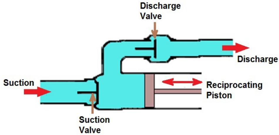
Figure 14: Schematic of a simple positive displacement pump.
