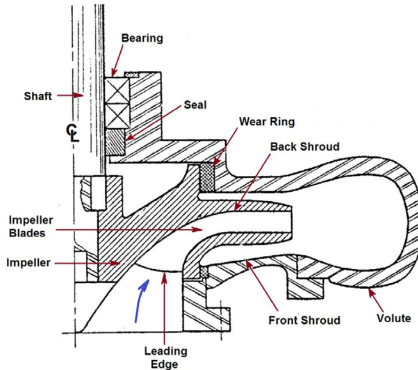
Figure 4: Components of a typical centrifugal pump.
