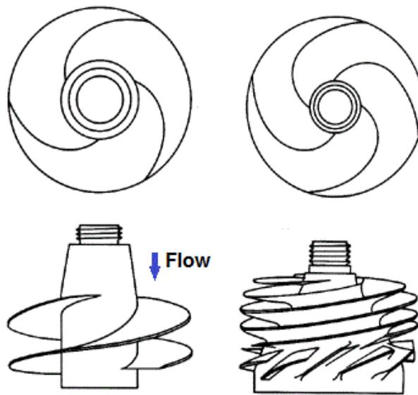
Figure 8: Two cavitating inducers: on the left a 9° helical inducer; on the right a scale model of the impeller in the SSME low pressure LOX turbopump.
