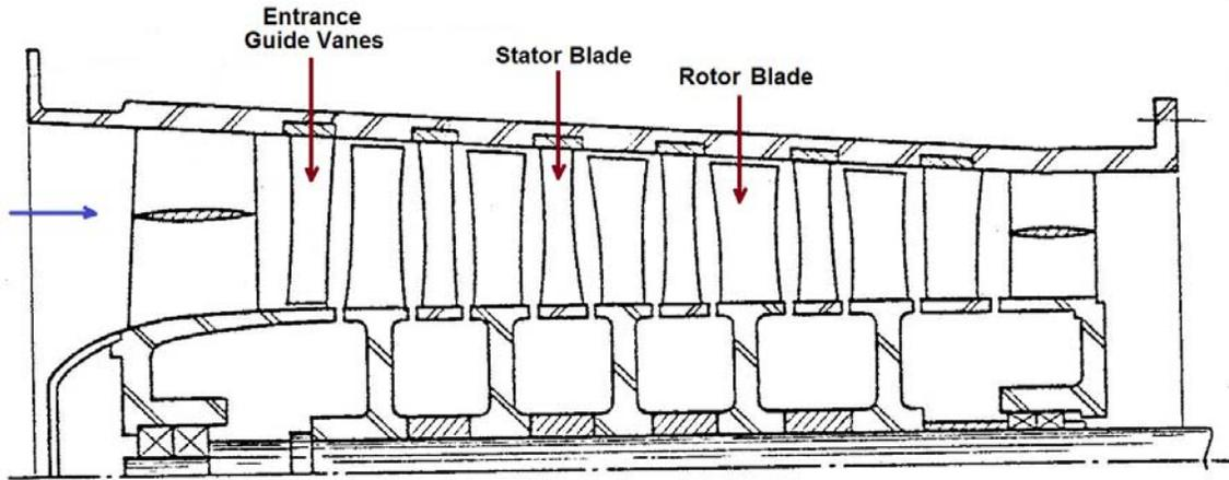
Figure 13: Typical axial compressor.
