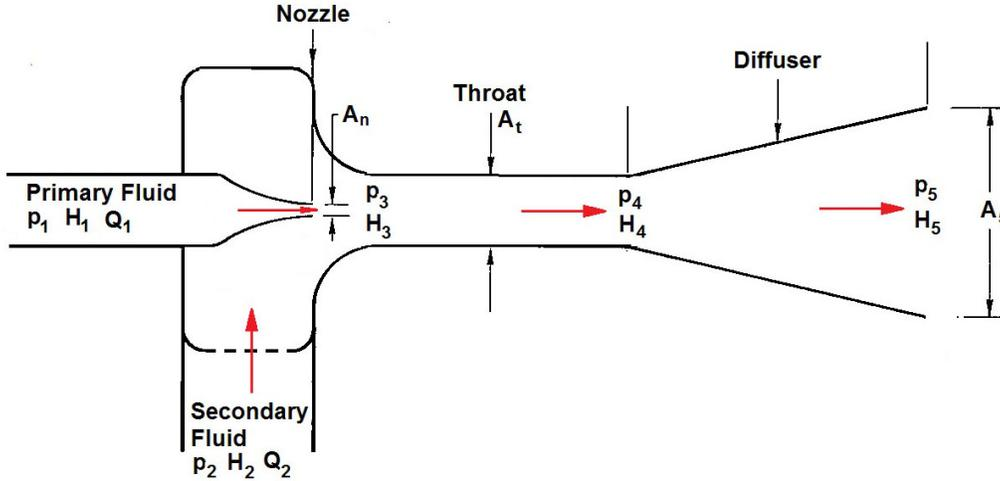
Figure 1: Basic jet pump geometry and notation.
