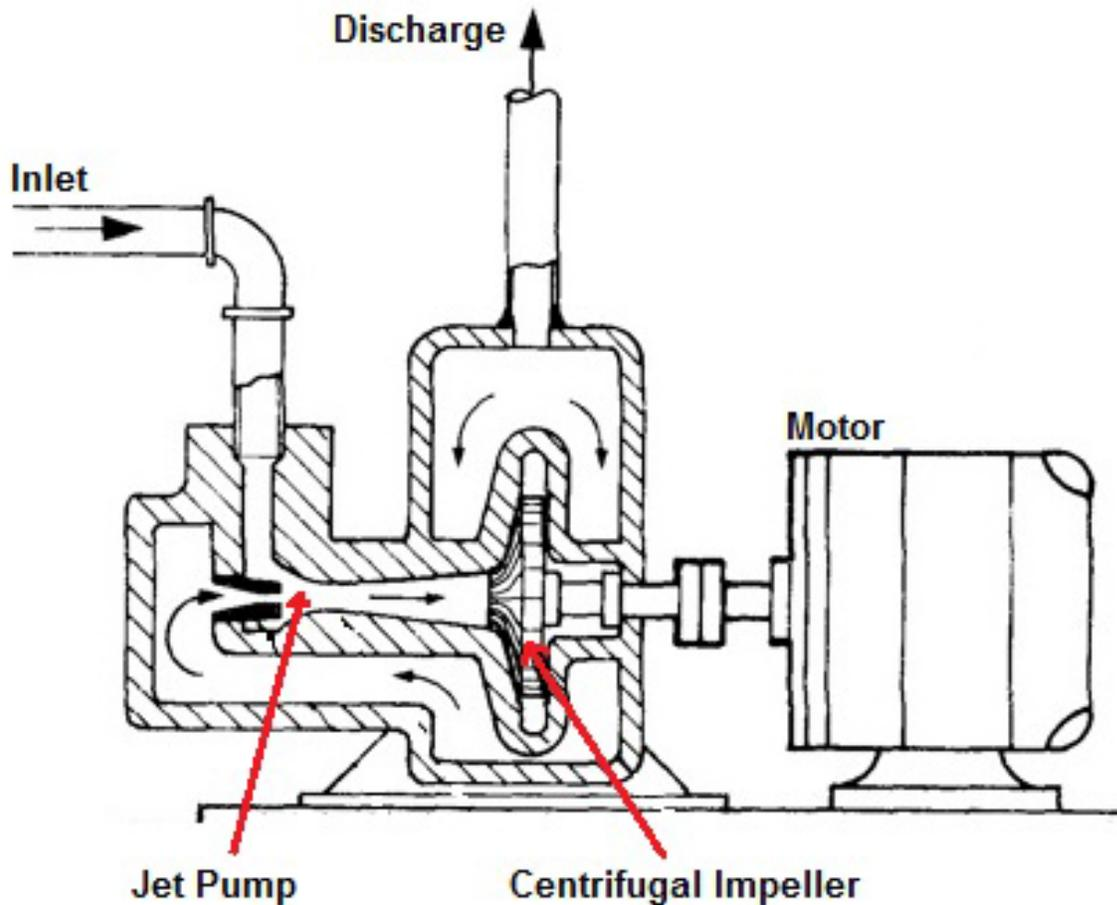
Figure 4: A typical combination of a jet pump with a centrifugal pump.
