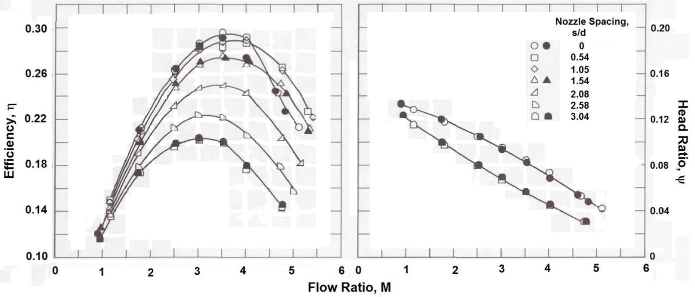
Figure 3: Typical jet pump performance curves from Sanger (1968a, 1968b): the head ratio,  $\psi$ , and efficiency,  $\eta$ , as a function of the flow ratio,  $M$ , for various relative locations of the nozzle ( $s/d$ ) and two different flow rates (open and closed symbols).
