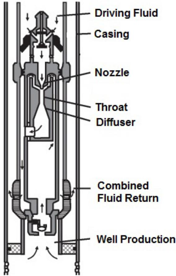
Figure 2: A deep oil well installation incorporating a jet pump. Adapted from Lea, Nickens and Wells (2008).
