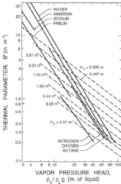
Figure 6: The parameter,  $B'$  (in  $m^{-1}$ ), for several liquids and  $H_T$  (in  $m$ ) for centrifugal pumps operating at design flow rate and at a 3% head drop (adapted from Knapp *et al.* 1970 and Stepanoff 1964).
