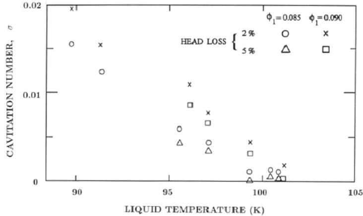
Figure 3: Effect of temperature on the cavitation performance of the J-2 liquid oxygen inducer pump (adapted from Gross 1973).
