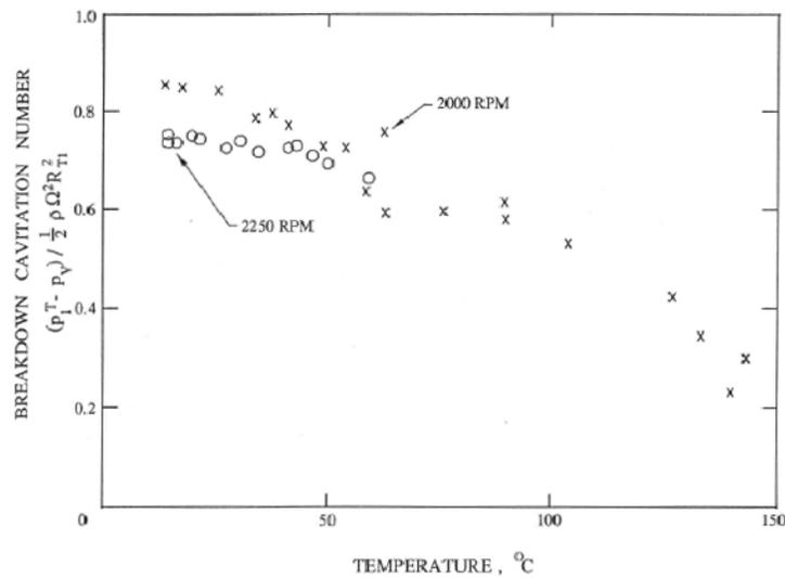
Figure 2: Thermodynamic effect on cavitation breakdown for a commercial centrifugal pump (data from Chivers 1969).
