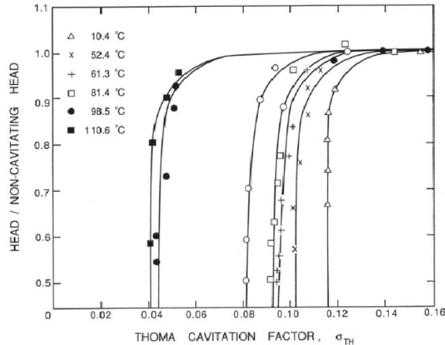
Figure 1: Typical cavitation performance characteristics for a centrifugal pump pumping water at various temperatures as indicated (Arndt 1981 from Chivers 1969).
