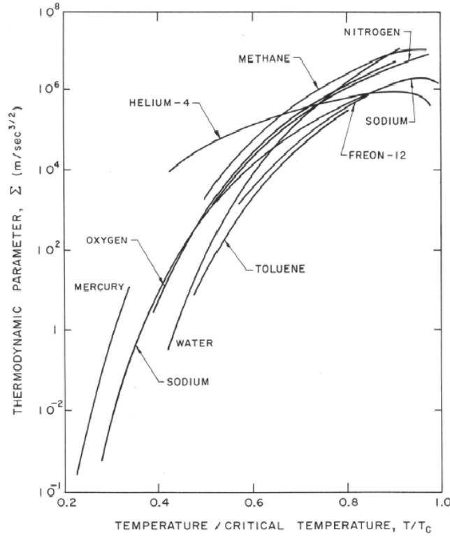
Figure 4: Thermodynamic parameter,  $\Sigma$ , as a function of temperature for various saturated fluids.
