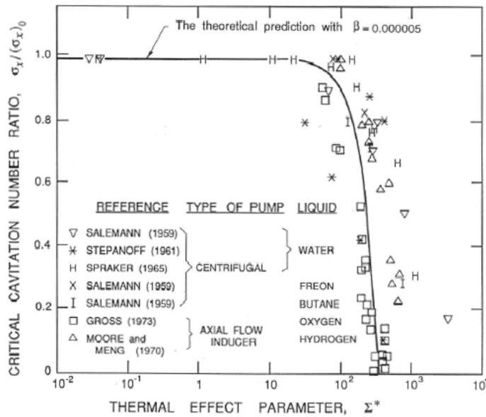
Figure 5: The ratio of the critical cavitation number  $\sigma_x$  ( $\sigma_a$  or  $\sigma_b$ ) to  $(\sigma_x)_0$  (the value of  $\sigma_x$  in the absence of any thermal effect) as a function of the thermal effect parameter,  $\Sigma^*$ . Data is shown for a variety of pumps and liquids.
