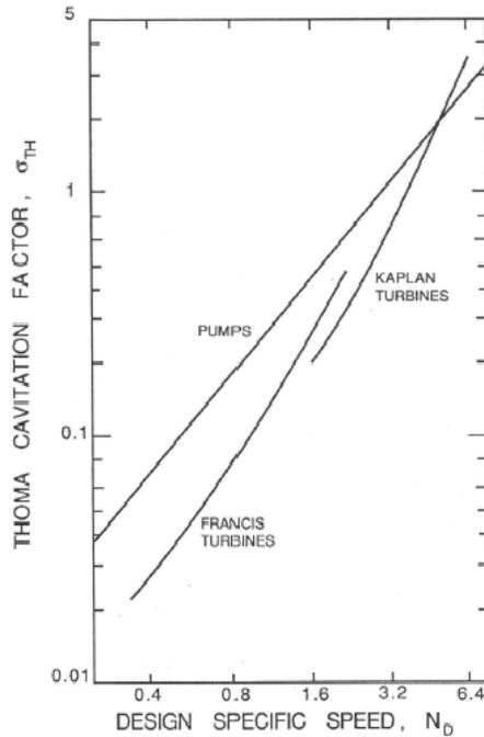
Figure 2: The Hydraulic Institute standards for the operation of pumps and turbines (Hydraulic Institute 1965).
