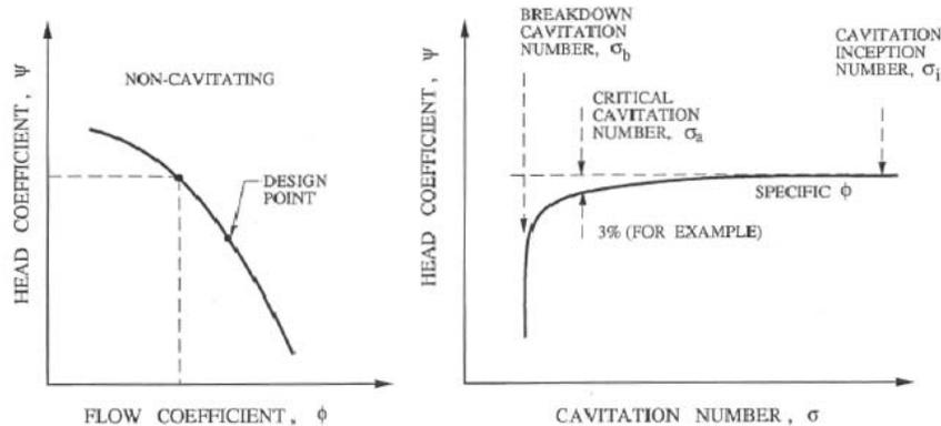
Figure 1: Schematic of noncavitating performance,  $\psi(\phi)$ , and cavitating performance,  $\psi(\phi, \sigma)$ , showing the three key cavitation numbers.
