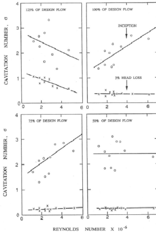
Figure 3: Inception and 3% head loss cavitation numbers plotted against a Reynolds number (based on  $w_{T1}$  and blade chord length) for four flow rates (from McNulty and Pearsall 1979).
