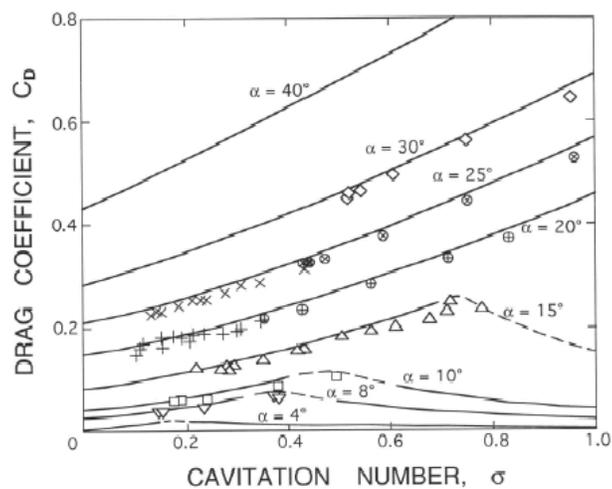
Figure 3: Drag coefficients corresponding to the lift coefficients of figure 2.
