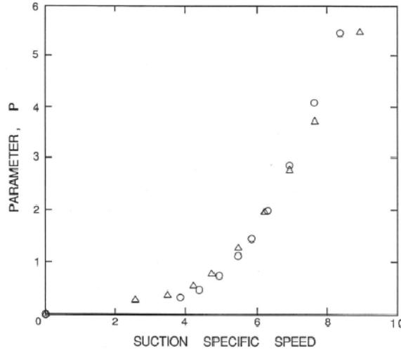
Figure 1: Some data on the cavitation head loss parameter,  $P = \Delta H/NPSH$ , for axial inducer pumps. The two symbols are for two different pumps.
