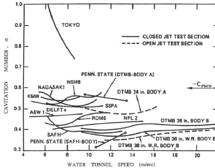
Figure 1: The inception numbers measured for the same axisymmetric headform in a variety of water tunnels around the world. Data collected as part of a comparative study of cavitation inception by the International Towing Tank Conference (Lindgren and Johnsson 1966, Johnsson 1969).
