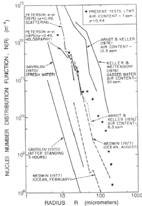
Figure 2: Several nuclei number distribution functions measured in water tunnels and in the ocean by various methods (adapted from Gates and Acosta 1978).
