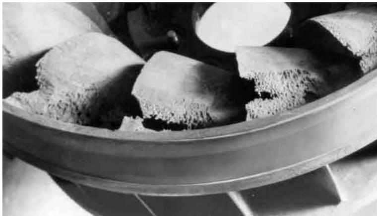
Figure 2: Cavitation damage on the blades at the discharge from a Francis turbine.
