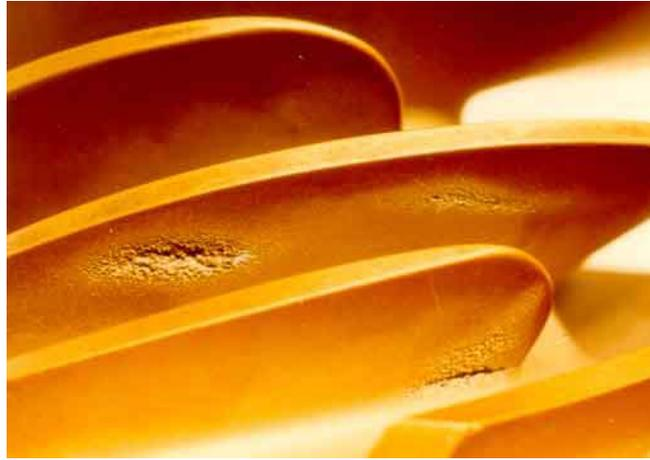
Figure 1: Photograph of localized cavitation damage on the blade of a mixed flow pump impeller made from an aluminium-based alloy.
