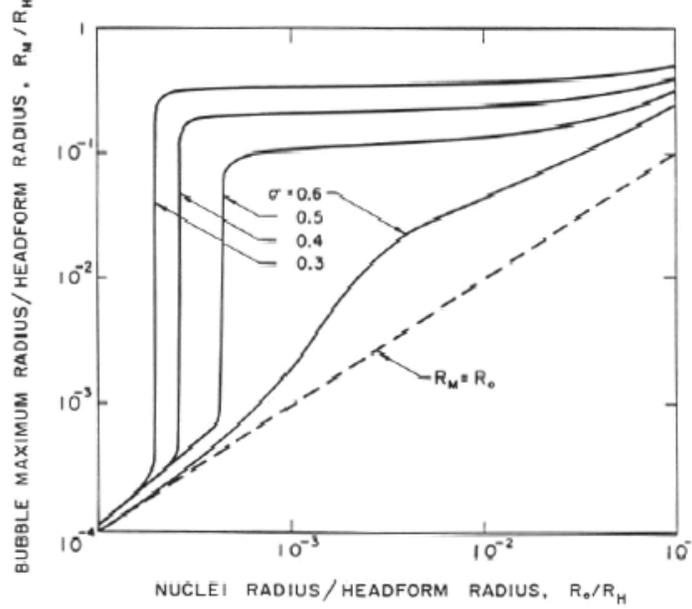
Figure 2: The maximum size to which a cavitation bubble grows (according to the Rayleigh-Plesset equation),  $R_M$ , as function of the original nuclei size,  $R_0$ , and the cavitation number,  $\sigma$ , in the flow around an axisymmetric headform of radius,  $R_H$ , with  $S/\rho_L R_H U^2 = 0.000036$  (from Ceccio and Brennen 1991).
