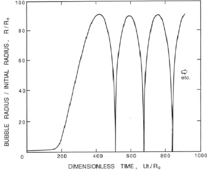
Figure 1: Typical solution,  $R(t)$ , of the Rayleigh-Plesset equation for a spherical bubble originating from a nucleus of radius,  $R_0$ . The nucleus enters a low pressure region at a dimensionless time of 0 and is convected back to the original pressure at a dimensionless time of 500. The low pressure region is sinusoidal and symmetric about a dimensionless time of 250.
