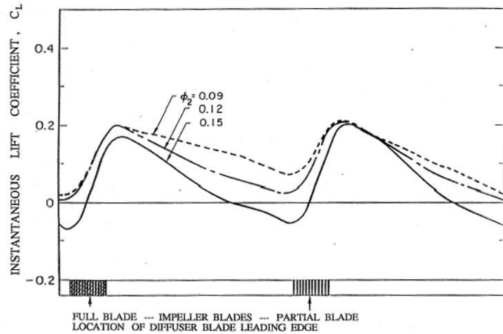
Figure 3: Variation in the instantaneous lift coefficient for a diffuser blade. The position of the diffuser blade leading edge relative to the impeller blade trailing edge is also shown. The data is for an interblade spacing of 4.5% (from Arndt *et al.* 1989).
