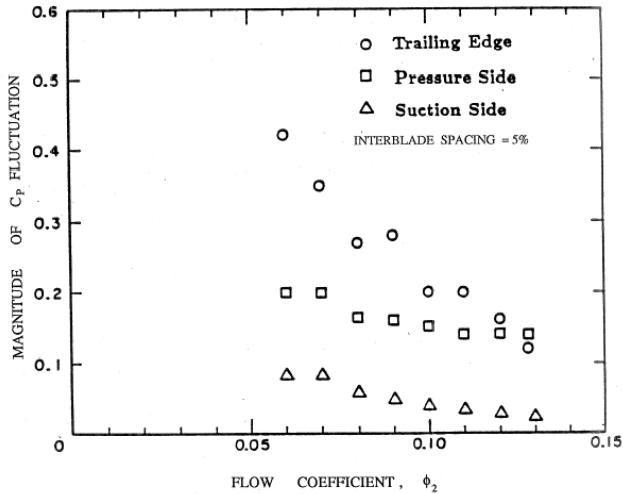
Figure 4: Magnitude of the fluctuations in the pressure coefficient at three locations near the trailing edge of an impeller blade during the passage of a diffuser blade (from Arndt *et al.* 1990).
