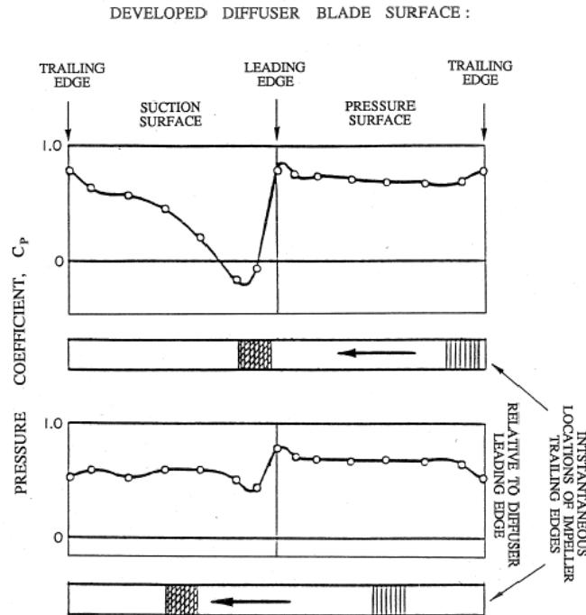
Figure 1: Pressure distributions on a diffuser blade at two different instants during the passage of an impeller blade. Data for an interblade spacing of 1.5% and  $\phi_2 = 0.12$  (from Arndt *et al.* 1989).
