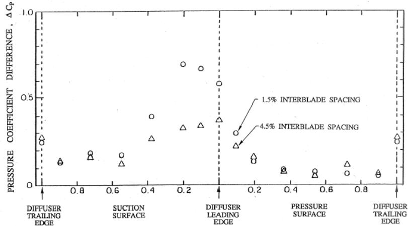
Figure 2: Magnitude of the fluctuation in the coefficient of pressure on a diffuser blade during the passage of an impeller blade as a function of location on the diffuser blade surface for two interblade spacings (from Arndt *et al.* 1989).
