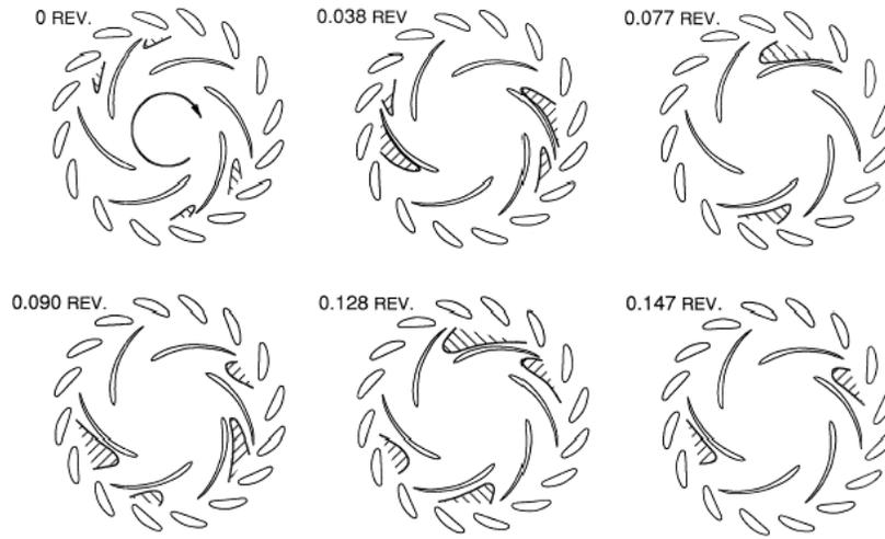
Figure 3: The propagation of a low pressure region (hatched) at nine times the impeller rotational speed in the flow through a high head pump-turbine. The sketches show six instants in time equally spaced within one sixth of a revolution. Made from videotape provided by Miyagawa *et al.* (1992).
