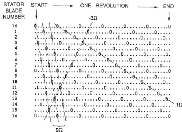
Figure 2: Encounter diagram for rotor-stator interaction in a turbomachine with  $Z_R = 6$ ,  $Z_S = 16$ .
