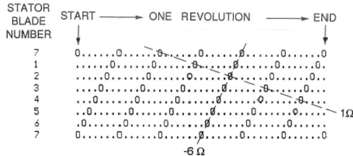
Figure 1: Encounter diagram for rotor-stator interaction in a turbomachine with  $Z_R = 6$ ,  $Z_S = 7$ . Each row is for a specific stator blade and time runs horizontally covering one revolution as one proceeds from left to right. Encounters between a rotor blade and a stator blade are marked by a 0.
