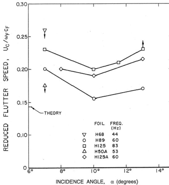
Figure 2: Dimensionless critical flutter speeds for single supercavitating hydrofoils at various angles of incidence,  $\alpha$ , and very long cavities ( $> 5$  chord lengths) (from Brennen, Oey, and Babcock 1980).
