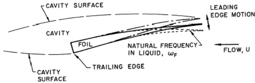
Figure 1: Sketch of the leading edge flutter of a cavitating hydrofoil or pump blade.
