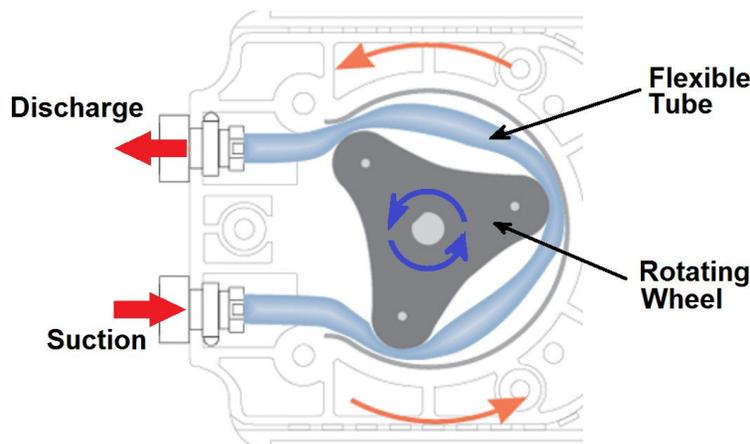
Figure 2: Schematic of a typical peristaltic pump.
