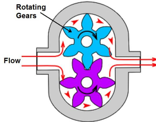
Figure 3: Schematic of a typical gear pump.
