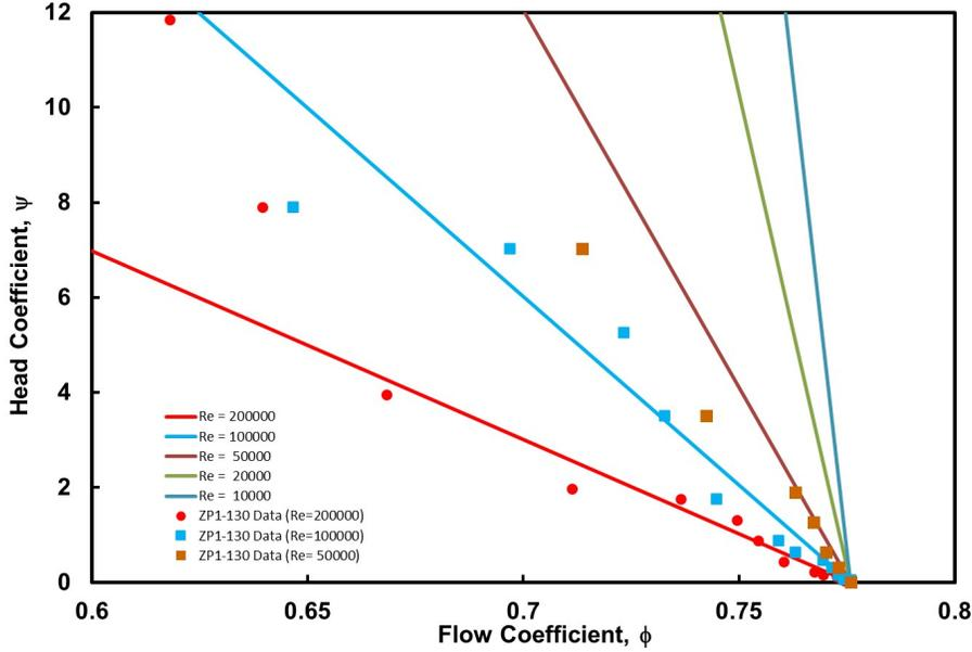
Figure 5: Non-dimensional performance of the AMPCO ZP1-130 positive displacement pump. The data points for three different Reynolds numbers were derived from dimensional information presented in the AMPCO webpage. The lines are the theoretical performance curves from equation (Mbj6) for five different Reynolds numbers as indicated.
