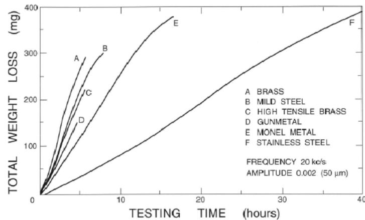
Figure 2: Examples of cavitation damage weight loss as a function of time. Data from vibratory tests with different materials (Hobbs, Laird and Brunton 1967).
