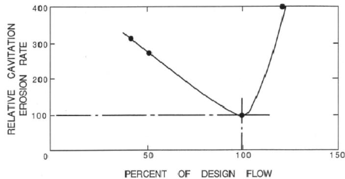
Figure 3: Cavitation erosion rates in a centrifugal pump as a function of the flow rate relative to the design flow rate (Pearsall 1978 from Grist 1974).
