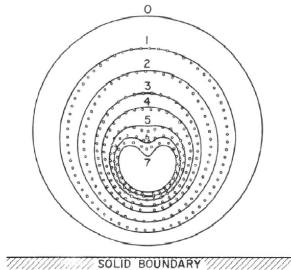
Figure 1: The collapse of a cavitation bubble close to a solid boundary. The theoretical shapes of Plesset and Chapman (1971) (solid lines) are compared with the experimental observations of Lauterborn and Bolle (1975) (points) (adapted from Plesset and Prosperetti 1977).
