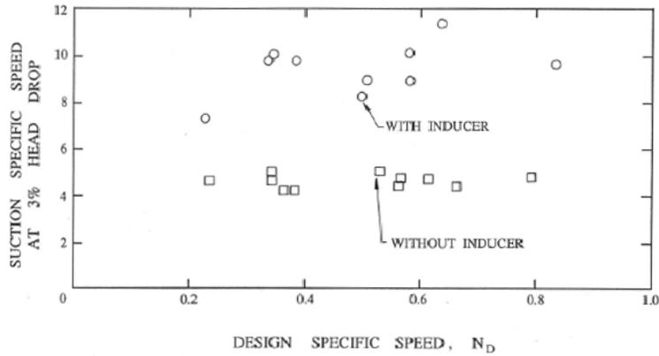
Figure 1: Comparison of the suction specific speed at 3% head drop for process pumps with and without inducer (from Janigro and Ferrini 1973).
