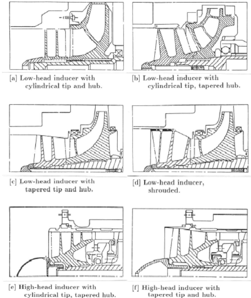
Figure 2: Various geometries of cavitating inducers (from Jakobsen 1971).
