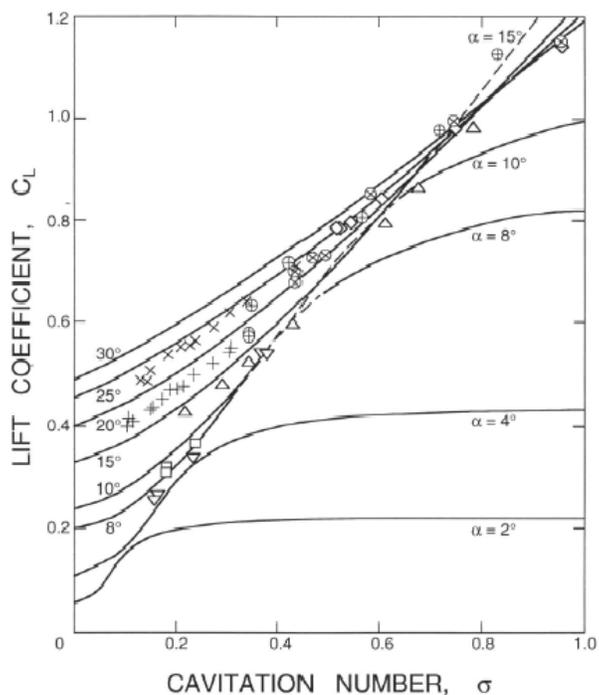
Figure 2: Lift coefficients for a flat plate from the non-linear theory of Wu (1962). The experimental data (Parkin 1958) is for angles of incidence as follows:  $8^\circ$  ( $\nabla$ ),  $10^\circ$  ( $\square$ ),  $15^\circ$  ( $\triangle$ ),  $20^\circ$  ( $\oplus$ ),  $25^\circ$  ( $\otimes$ ), and  $30^\circ$  ( $\diamond$ ). Also shown is some data of Silberman (1959) in a free jet tunnel:  $20^\circ$  ( $+$ ) and  $25^\circ$  ( $\times$ ).
