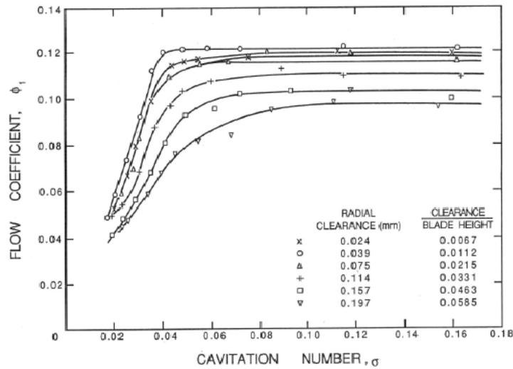
Figure 3: The effect of tip clearance on the cavitation performance of a cavitating inducer (from Henderson and Tucker 1962 as given by Janigro and Ferrini 1973).
