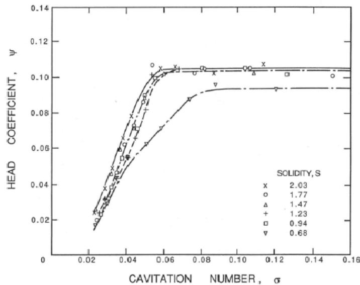
Figure 2: The effect of solidity on the cavitation performance of a cavitating inducer (Janigro and Ferrini 1973 from Henderson and Tucker 1962).
