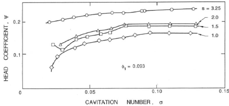
Figure 1: The effect of solidity on the cavitation performance of a  $9^\circ$  helical inducer (from Acosta 1958).
