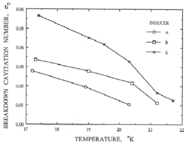
Figure 5: The breakdown cavitation numbers,  $\sigma_b$  (defined in this case by a 30% head drop) as a function of temperature for three shapes of leading edge (see figure 4) on  $9.4^{\circ}$  helical inducers operating in liquid hydrogen (from Moore and Meng 1970a,b).
