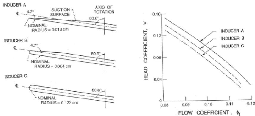
Figure 4: Non-cavitating performance of three 9.4° helical inducers with different leading edges as shown. Tests performed with liquid hydrogen (from Moore and Meng 1970b).
