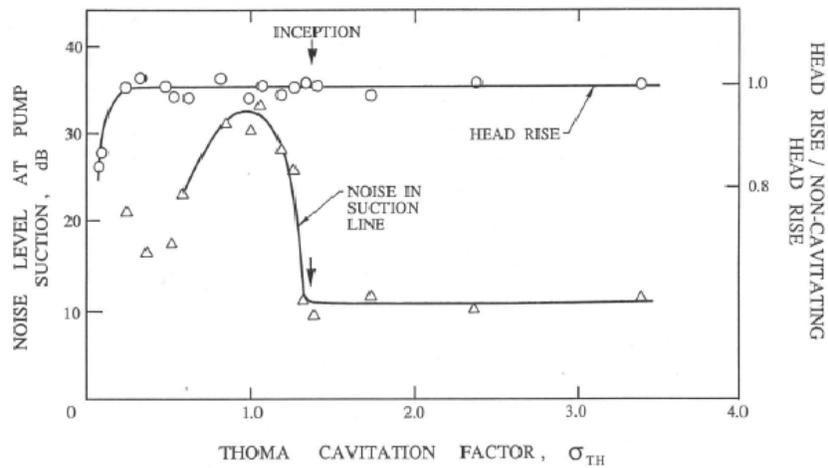
Figure 2: Head rise and suction line noise as a function of the Thoma cavitation factor,  $\sigma_{TH}$ , for a typical centrifugal pump (adapted from McNulty and Pearsall 1979).
