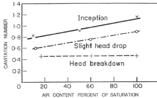
Figure 3: The effect of air content on the critical cavitation numbers for a centrifugal pump (Schoeneberger 1965, Pearsall 1972).
