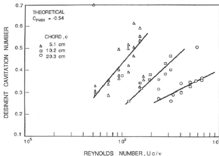
Figure 7: The desinent cavitation numbers for three geometrically similar Joukowski hydrofoils at zero angle of incidence as a function of Reynolds number,  $Uc/\nu$  (Holl and Wislicenus 1961). Note the theoretical  $C_{pmin} = -0.54$ .
