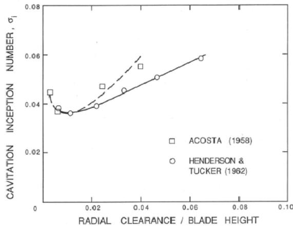
Figure 9: The cavitation inception number as a function of radial tip clearance in an axial inducer (Janigro and Ferrini 1973 from data of Acosta 1958 and Henderson and Tucker 1962).
