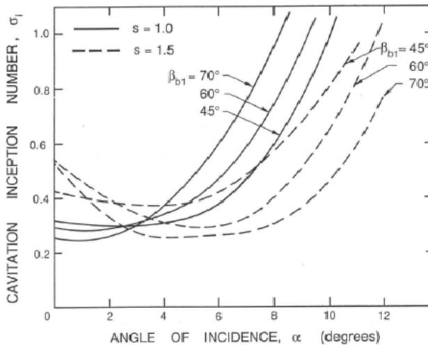
Figure 5: Calculated cavitation inception number,  $\sigma_i$  (or  $-C_{pmin}$ ), as a function of blade angle,  $\beta_{b1}$ , solidity,  $s$ , and incidence angle,  $\alpha$ , for a cascade of NACA-65-010 hydrofoils (Herrig *et al.* 1957, Pearsall 1972).
