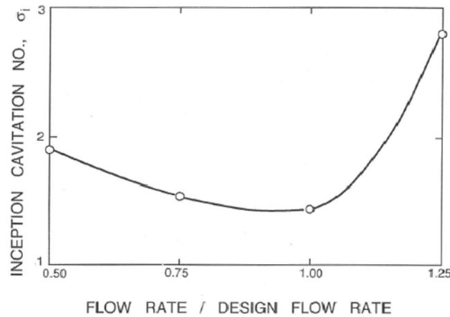
Figure 6: Variation in the inception number with flow rate for a typical centrifugal pump (adapted from McNulty and Pearsall 1979).
