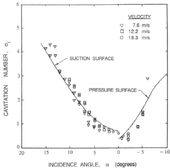
Figure 4: Cavitation inception characteristics of a NACA 4412 hydrofoil (Kermeen 1956).
