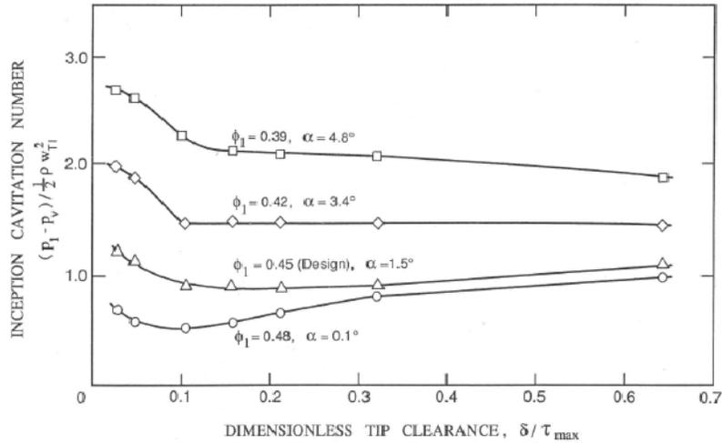
Figure 8: The cavitation inception number,  $\sigma_i$ , as a function of tip clearance,  $\delta$  ( $\tau_{max}$  is the maximum blade thickness), in an unshrouded axial flow pump at various flow coefficients,  $\phi$  (adapted from Rains 1954).
