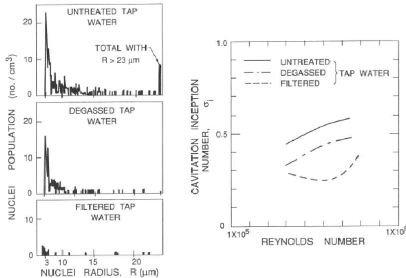
Figure 1: Histograms of nuclei populations in treated and untreated tap water and the corresponding cavitation inception numbers on hemispherical headforms of three different diameters (Keller 1974).
