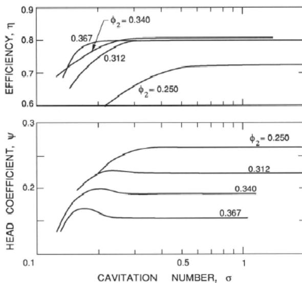
Figure 9: Effect of cavitation on the head coefficient and efficiency of one of the axial flow pumps of figure 4. The cavitation number is based on  $w_{T1}$ . Adapted from Oshima and Kawaguchi (1963).
