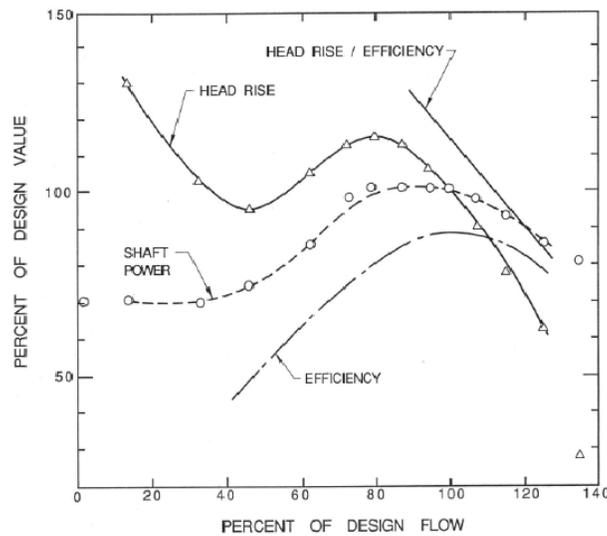
Figure 5: Characteristics of a mixed flow pump (Myles 1966).
