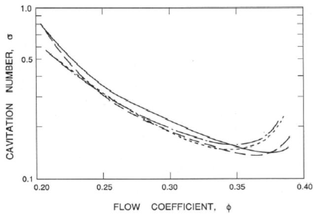
Figure 10: The critical cavitation number (based on  $w_{T1}$  and 0.5% head loss) for the axial flow pumps of figure 4. Adapted from Oshima and Kawaguchi (1963).
