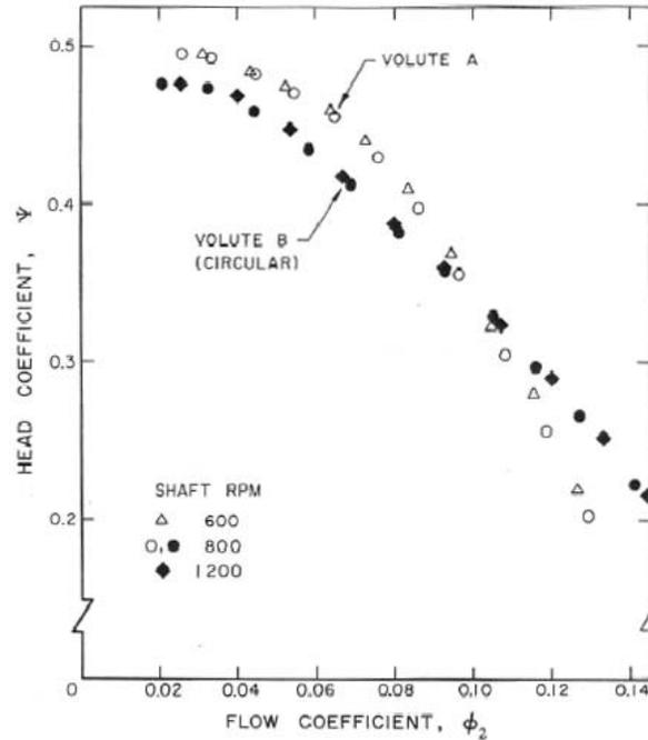
Figure 1: Typical non-cavitating performance for a centrifugal pump, namely Impeller X (see section (Mbbi)) with Volute A and a circular volute of uniform cross-section (from Chamieh 1983).
