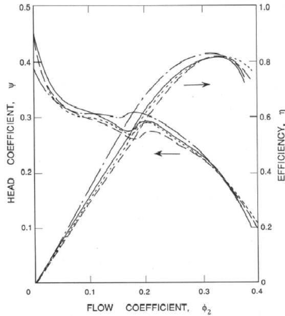
Figure 4: Typical non-cavitating performance characteristics for a four-bladed axial flow pump with tip blade angle,  $\beta_{bT}$ , of about  $18^\circ$ , a hub-tip ratio,  $R_H/R_T$ , of 0.483, a solidity of 0.68 and four different blade profiles (yielding the set of four performance curves). Adapted from Oshima and Kawaguchi (1963).
