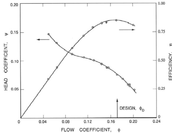
Figure 3: Typical non-cavitating performance characteristics for a 20.3cm diameter, 3-bladed axial flow pump with a hub-tip ratio,  $R_H/R_T$ , of 0.45 running at about 1500rpm. At the blade tip the chord is 7.3cm, the solidity is 0.344 and the blade angle,  $\beta_{iT}$ , is  $11.9^\circ$ . Adapted from Guinard *et al.* (1953).
