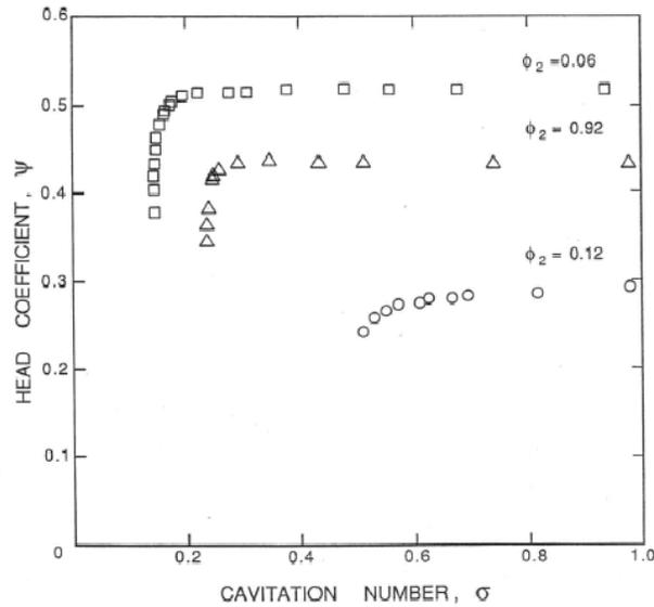
Figure 2: Cavitation performance for the Impeller X/Volute A combination (from Franz *et al.* 1989, 1990). The flow separation rings of figure ?? have been installed so the non-cavitating performance is slightly better than in figure 1.
