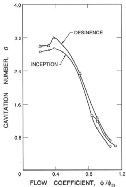
Figure 8: Inception and desinent cavitation numbers (based on  $w_{T1}$ ) as a function of  $\phi/\phi_D$  for the axial flow pump of figures 3 and 7. Adapted from Guinard *et al.* (1953).
