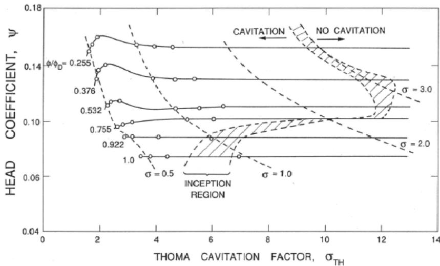
Figure 7: Cavitation performance characteristics of the axial flow pump of figure 3. Adapted from Guinard *et al.* (1953).
