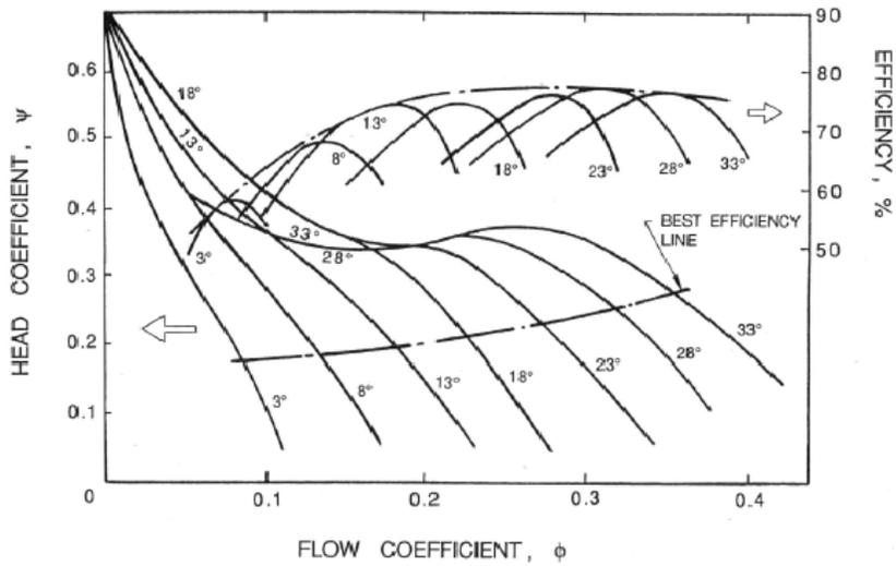
Figure 6: Head and efficiency characteristics for an axial flow pump with different tip blade angles,  $\beta_{bT}$  (from Peck 1966).
