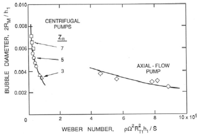
Figure 1: The bubble diameters observed in the blade passages of centrifugal and axial flow pumps as a function of Weber number (adapted from Murakami and Minemura 1978).
