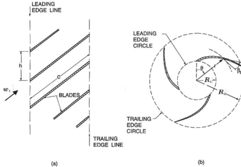
Figure 1: Schematics of (a) a linear cascade and (b) a radial cascade.
