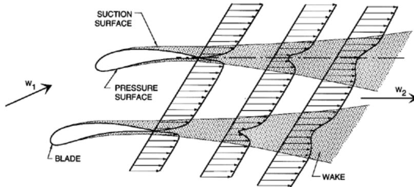
Figure 1: Sketch of the boundary layers on the surfaces of a cascade and the resulting blade wakes.
