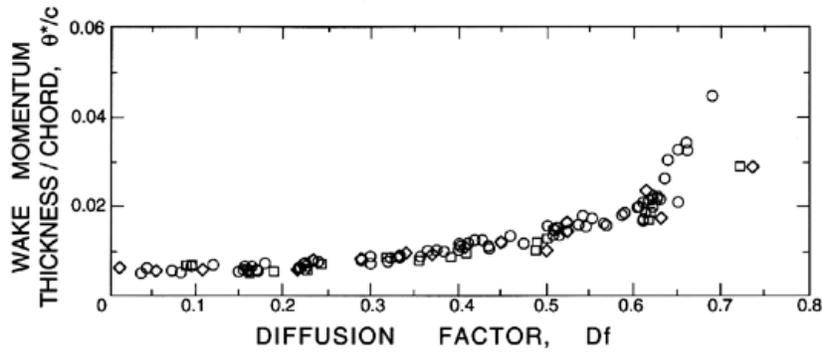
Figure 2: Correlation of the ratio of the momentum thickness of the blade wakes,  $\theta^*$ , to the chord,  $c$ , with the diffusion factor,  $Df$ , for cascades of blades with three different profiles: NACA 65 – ( $A_{10}$ )10 series ( $\circ$ ) and two British C.4 parabolic arc profiles ( $\square$  and  $\diamond$ ). The maximum thickness of the blades is  $0.1c$  and the Reynolds number is  $2.5 \times 10^5$ . Adapted from Lieblein (1965).
