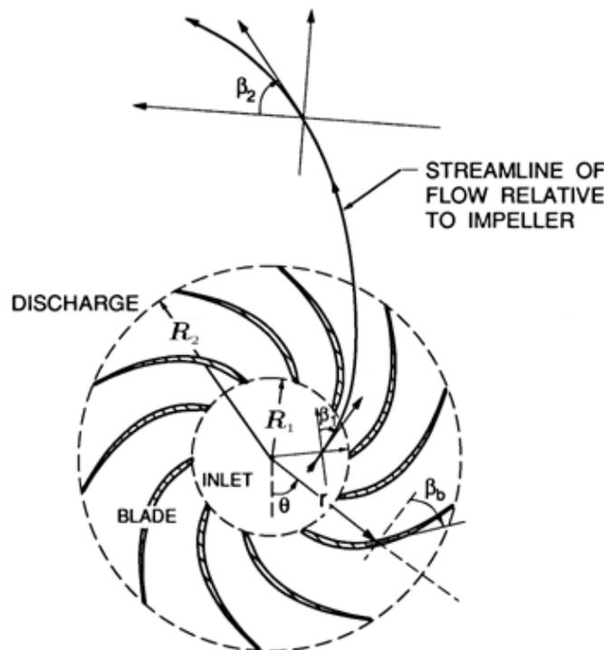
Figure 1: Schematic of the radial cascade corresponding to the linear cascade of figure ??.
