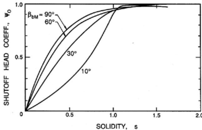
Figure 1: The performance parameter,  $\psi_0$ , as a function of solidity,  $s$ , for flat plate cascades with different blade angles,  $\beta_b$ . Adapted by Wislicensus (1947) (see also Sabersky, Acosta and Hauptmann 1989) from the potential flow theory of König (1922).
