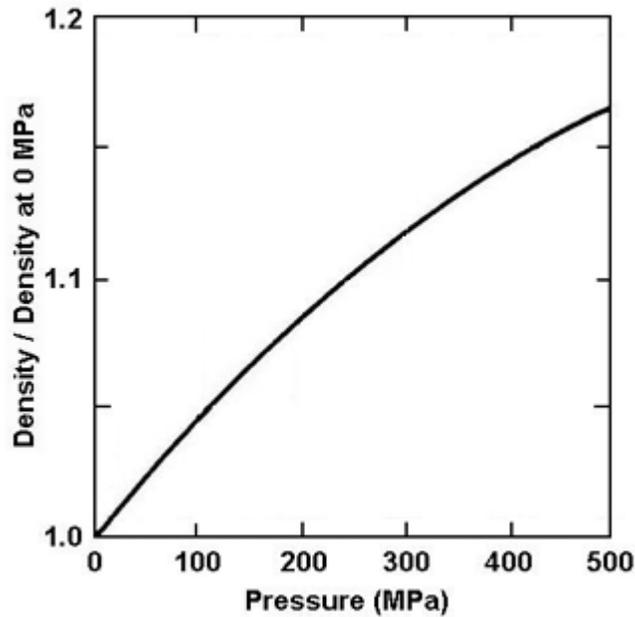
Figure 2: The variation in the density of water with pressure at  $0^{\circ}\text{C}$ .
