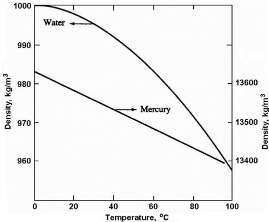
Figure 1: The density of water and mercury as a function of temperature at a pressure of one atmosphere.
