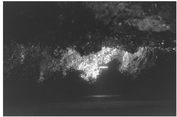
Fig. 6 Photograph of bubble clouds passing by the IVFM probe, the tip of which is visible in the center. The flow is from right to left with \theta = 25^\circ , \phi = 0^\circ , U = 2.47 m/s, d = 7.39 cm, and F = 2.90 .
