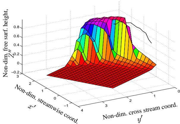
**FIGURE 13: Non-dimensional water surface topography along with the contact line from a larger scale experiment;  $\theta = 26.6^\circ$ ,  $\phi = 0^\circ$ ,  $U = 2.39\text{m/s}$ ,  $d = 7.56\text{cm}$ , AND  $\mathbf{F} = 2.77$ . The leading edge of the deflecting plate is located at  $(x', y') = (0, 0)$ .**
