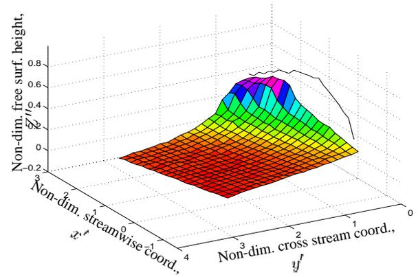
**FIGURE 12: Non-dimensional water surface topography along with the contact line from a larger scale experiment;  $\theta = 13.4^\circ$ ,  $\phi = 0^\circ$ ,  $U = 2.43\text{m/s}$ ,  $d = 7.56\text{cm}$ , and  $\mathbf{F} = 2.81$ . The leading edge of the deflecting plate is located at  $(x', y') = (0, 0)$ .**
