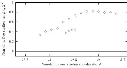
(a) Jet cross-section at non-dim. stream-wise coordinate,  $x' = 3.46$
