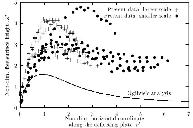
**FIGURE 9: Comparison of the non-dimensional profiles of the bow wave along the deflecting plate from the smaller scale and the larger scale experiments. Ogilvie's analytical profile is shown as a solid black line.**
