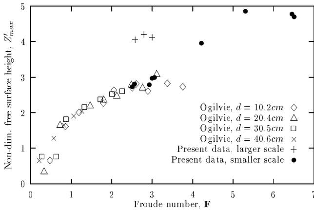
**FIGURE 10: Comparison of the  $\theta = 13.4^\circ$  smaller scale ( $d = 1.4\text{cm}$ ) and larger scale ( $d \approx 7.8\text{cm}$ ) experimental results to Ogilvie's  $\theta = 15^\circ$  experimental results.**
