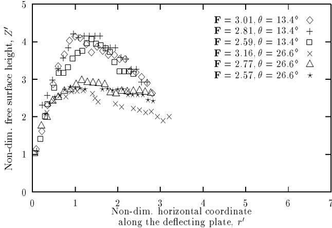
**FIGURE 8: Non-dimensional profiles of the bow wave along the deflecting plate from larger scale experiments with two different angles  $\theta$ .**
