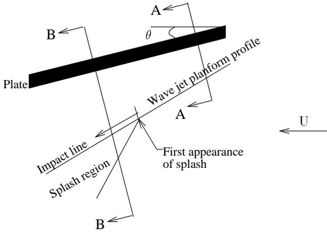
**FIGURE 2: Schematic diagram of the flow features.**
