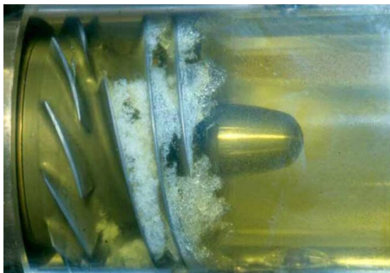
Fig. 5 (Color online) Cavitating model of the Low Pressure Liquid Oxygen Pump in the Space Shuttle Main Engine [13]
