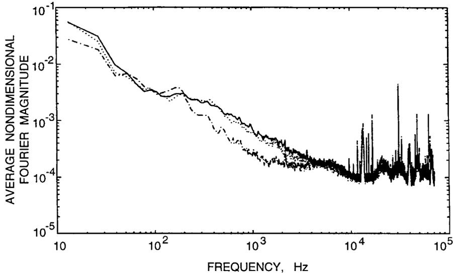
**FIGURE 3:** Effect of air injection on the spectral content of the noise for three normalized air flow rates. Data is from the NACA 64A309 foil with  $k = 0.8$ ,  $\sigma = 1.2$ ,  $\bar{\alpha}_f = 9^\circ$ ,  $U = 8m/s$ , an air content of  $7 - 10ppm$ ,  $q = 1.3 \times 10^{-4}$  (—),  $q = 2.4 \times 10^{-4}$  (····), and  $q = 9.8 \times 10^{-4}$  (-·-·-·).
