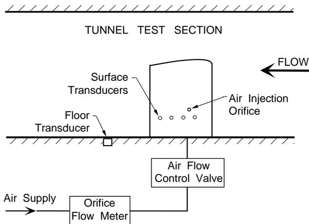
**FIGURE 1:** Sketch of the NACA 0021 foil and the air injection system.
