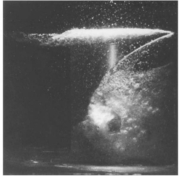
**FIGURE 5:** Visual effect of air injection on cloud cavitation. The photograph on the left is without air injection, the photograph on the right has a normalized air flow rate of  $q = 4.5 \times 10^{-4}$ . Both photographs are of the NACA 64A309 with  $k = 0.8$ ,  $\sigma = 1.2$ , and  $\alpha = 12.3^\circ$  ( $\alpha$  decreasing).
