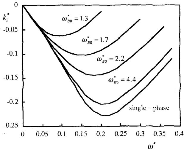
Figure 1. The attenuation rate ( $k_i^*$ ) as a function of the frequency,  $\omega^*$ , for a void fraction of  $\alpha = 0.005$  and various bubble natural frequencies:  $\omega_{B0}^* = 4.4$ ,  $\omega_{B0}^* = 2.2$ ,  $\omega_{B0}^* = 1.7$ , and  $\omega_{B0}^* = 1.35$ . Also shown is the single-phase flow result.
