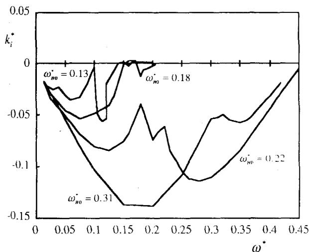
Figure 6. Data illustrating the effect of bubble resonant behavior ( $\omega^* = \omega_{B0}^*$ ). The attenuation rate ( $k_i^*$ ) is shown as a function of the perturbation frequency,  $\omega^*$ , for  $\omega_{B0}^* = 0.31$ ,  $\omega_{B0}^* = 0.22$ ,  $\omega_{B0}^* = 0.18$ , and  $\omega_{B0}^* = 0.14$ .
