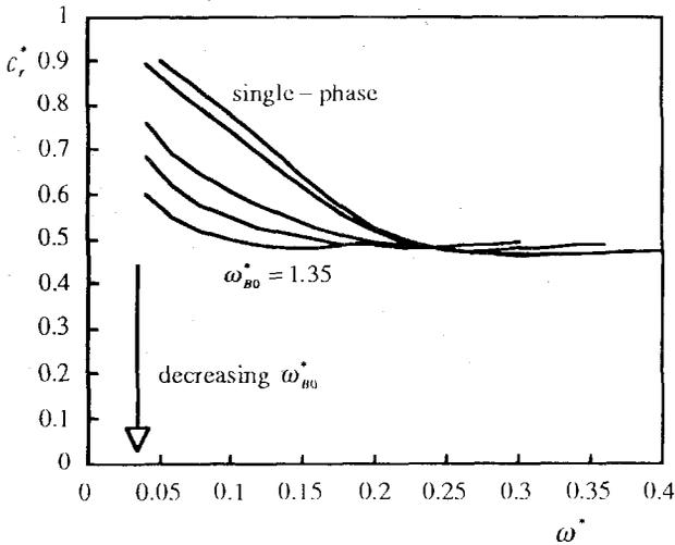
Figure 5. The phase velocity,  $c_r^*$ , as a function of the excitation frequency,  $\omega^*$ , for  $\omega_{B0}^* = 4.4$ ,  $\omega_{B0}^* = 2.2$ ,  $\omega_{B0}^* = 1.7$ , and  $\omega_{B0}^* = 1.35$ . Also shown is the single-phase flow result.
