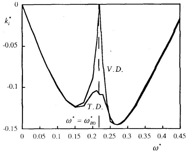
Figure 7. Data illustrating the effect of bubble damping. The attenuation rate ( $k_i^*$ ) as a function of the perturbation frequency,  $\omega^*$ , for bubble with total damping (T.D.) and bubble with only viscous damping (V.D.)
