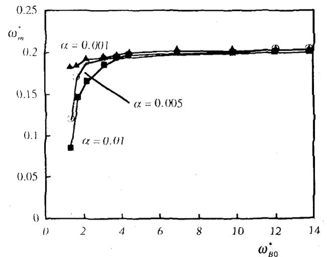
Figure 4. The frequency,  $\omega_m^*$ , corresponding to most unstable attenuation rate, as a function of the bubble natural frequency,  $\omega_{B0}^*$ , for  $\alpha = 0.001$ ,  $\alpha = 0.005$ , and  $\alpha = 0.01$ .
