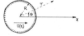
The resulting fluid velocities  $u_r u_v$  in the r and v directions are then given by a velocity potential,  $\varphi$ , such that
