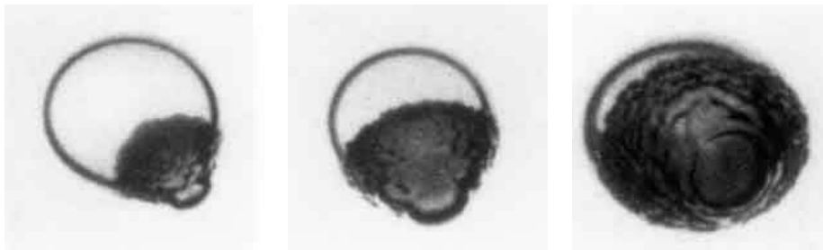
Figure 1: Typical photographs of a rapidly growing bubble in a droplet of superheated ether suspended in glycerine. The bubble is the dark, rough mass; the droplet is clear and transparent. The photographs, that are of different events, were taken 31, 44, and 58 \mu s after nucleation and the droplets are approximately 2 mm in diameter. Reproduced from Frost and Sturtevant (1986).
