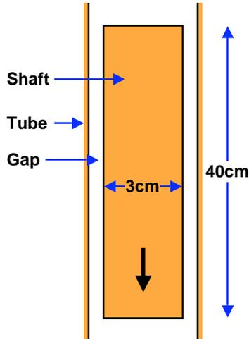
acceleration). In this particular problem, we will neglect the buoyancy force, because the weight of the shaft is much greater than the weight of the displaced fluid. The two forces on the shaft are thus the weight of the shaft itself and the viscous forces acting on the shaft’s cylindrical surface:
